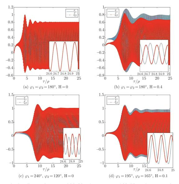
Fig. 6. Axial oscillations of symmetrical (a), (b) and nonsymmetrical (c), (d) angular position of cutters and for various cases of axial offset H as a function of nondimensional time  $\tau/\rho$ .
