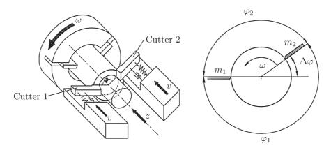
Fig. 2. Schematic of the two-cutter turning.
