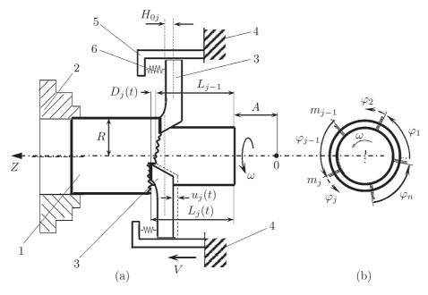
Fig. 1. Multiple cutter process model.
