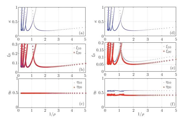
Fig. 4. Stability investigation for symmetrical cutter position ( $\alpha = 1$ ) with zero offset, i.e., H = 0 (a)–(c) and nonzero offset, i.e. H = 0.1 (d)–(f) for the case  $\eta_* = 0.1, r = 0.55, \varsigma = 0.05$ : stability lobe diagram (a), (d) and the steady cutter deflection (b), (e), steady chip thickness (c), (f).
