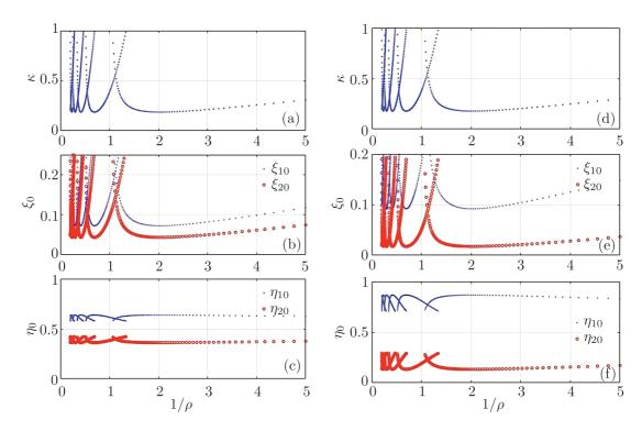
Fig. 5. Stability investigation for nonsymmetrical cutter position and zero axial shift, i.e.,  $\alpha = 2$ , H = 0 (a)–(c) and nonzero shift, i.e.,  $\alpha = 1.18$ , H = 0.4 (d)–(f) for the case  $\eta_* = 0.1$ , r = 0.55,  $\varsigma = 0.05$  stability lobe diagram (a), (d) and the steady cutter deflection (b), (e), steady chip thickness (c), (f).
