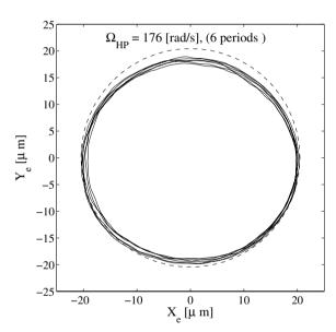
Fig. 8. Journal orbit at the 1st critical speed.
