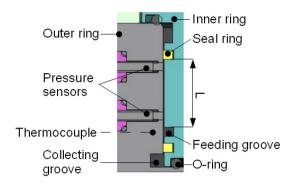
Fig. 3. Close-up view of the SFD, axial cross-section.
