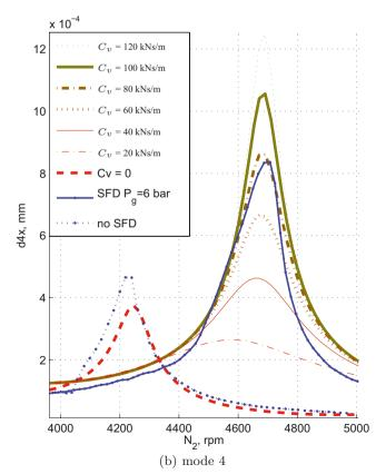
Fig. 6. Numerical and experimental unbalance response plot in view of estimation of apparent  $C_{\rm v}$  at the middle of LP shaft.
