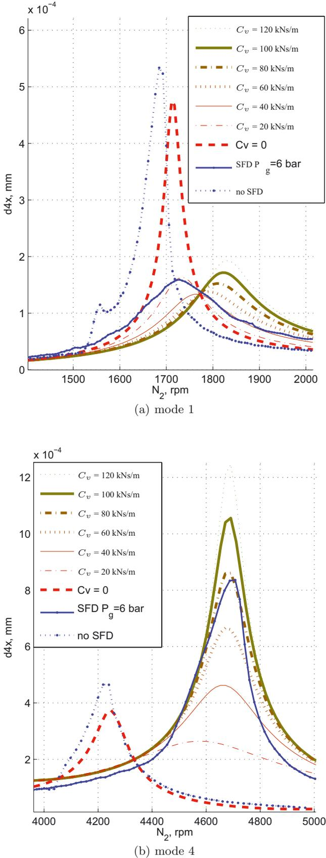
**Fig. 6.** Numerical and experimental unbalance response plot in view of estimation of apparent  $C_v$  at the middle of LP shaft.
