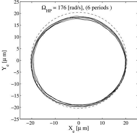
**Fig. 8.** Journal orbit at the 1st critical speed.
