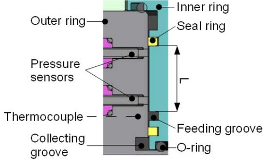
Fig. 3. Close-up view of the SFD, axial cross-section.
