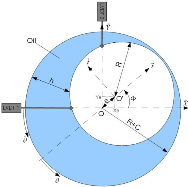
Fig. 4. Schematic of the SFD – transverse cross-section.
