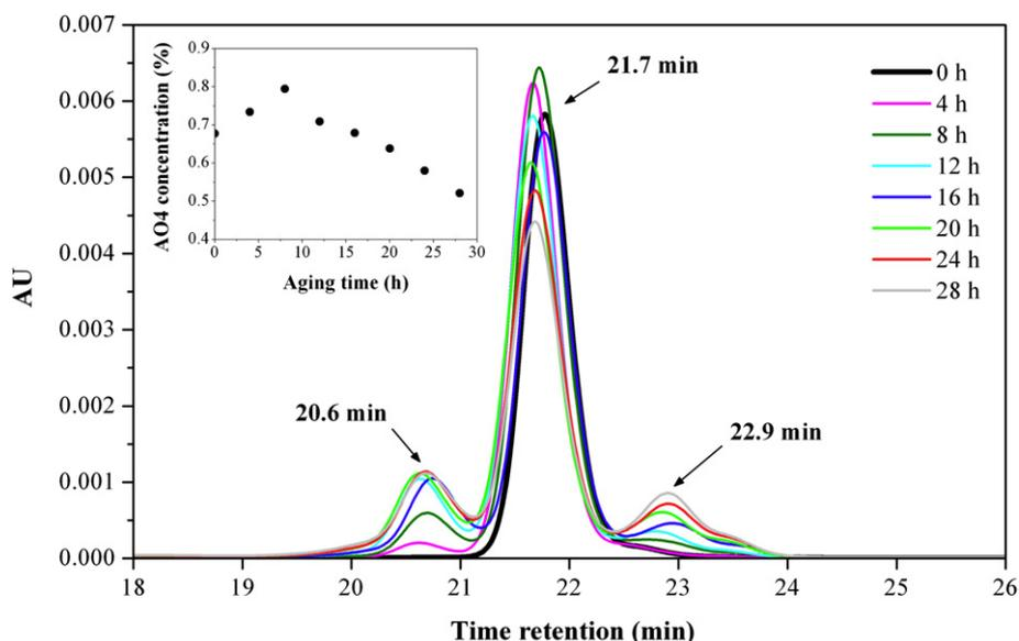
**Fig. 4.** Series GPC chromatograms of the AO4 antioxidant acquired at 276 nm after oxidation exposure at  $110 \text{ }^\circ\text{C}$  under 3.0 MPa oxygen pressure.
