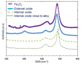
Fig. 5. Raman spectra of  $Fe_3O_4$  derived from the RRUFF database (ID #R060191) [27] and of a P sample exposed to hydrogenated SCW at 600 °C and 25 MPa.
