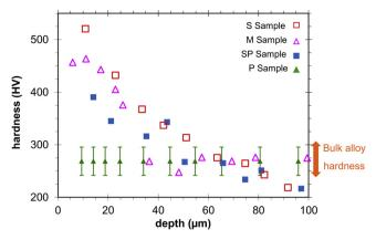
**Fig. 1.** Comparison of hardness profiles obtained from the studied surface states before corrosion tests for the P, M, S and SP samples. The standard error of hardness measurements is estimated statistically at approximately 10% from the experimental measurements.
