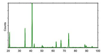
Fig. 4. XRD analyses performed in the  $\theta/2\theta$  mode on P sample exposed to hydrogenated SCW at 600 °C and 25 MPa for 335 h showing characteristics of magnetite Fe<sub>3</sub>O<sub>4</sub> from the external oxide.
