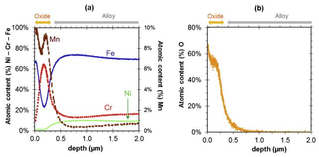
**Fig. 11.** Atomic composition profiles recorded *via* GDOS for an M sample exposed to hydrogenated SCW for 335 h at 600 °C and 25 MPa: a) Fe, Cr, Ni and Mn profiles (normalized to the total metallic elements at each point) and b) the corresponding O profile.
