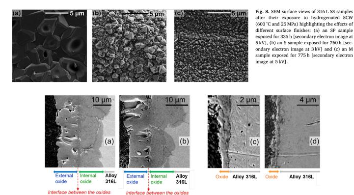
Fig. 9. SEM cross-section views of 316 L SS samples after their exposure to hydrogenated SCW (600 °C and 25 MPa) highlighting the effects of different surface finishes: (a) P and (b) SP samples exposed for 335 h, (c) an M sample exposed for 350 h and (d) an S sample exposed for 1010 h.
