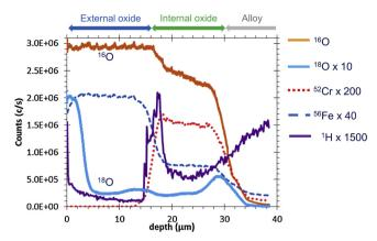
**Fig. 7.** H, O, Cr and Fe profiles obtained by SIMS applied to a P sample exposed to hydrogenated SCW (600 °C and 25 MPa) over a two-staged corrosion experiment (760 h in natural water followed by 308 h in water enriched with <sup>18</sup>O); intensities of <sup>1</sup>H, <sup>18</sup>O, <sup>52</sup>Cr and <sup>56</sup>Fe signals are multiplied respectively by 1500, 10, 200 and 40.
