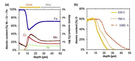
**Fig. 3.** Atomic composition profiles recorded by GDOS on P samples exposed to hydrogenated SCW at 600 °C and 25 MPa: a) Fe, Cr, Ni and Mn profiles (normalized with respect to the total number of metallic elements at each point) recorded after 335 h of exposure and b) O profiles recorded for exposure periods of 335 h to 3380 h.
