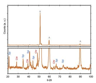
**Fig. 12.** XRD analysis performed in the  $\theta/2\theta$  mode on M sample exposed to hydrogenated SCW at 600 °C and 25 MPa for 335 h. The below pattern is focused on the oxide characteristics. The peaks corresponding to the chromia, a mixed spinel and the alloy are respectively indicated by Chr, Spi and A.
