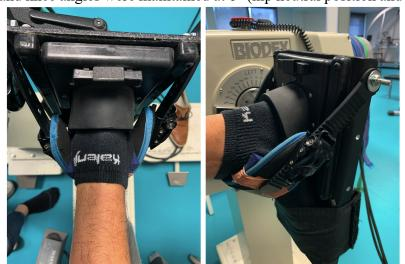
Figure 2: Modified ankle Biodex accessory. A snowboard binding was attached to the Biodex accessory to avoid any movement of the ankle and foot.
