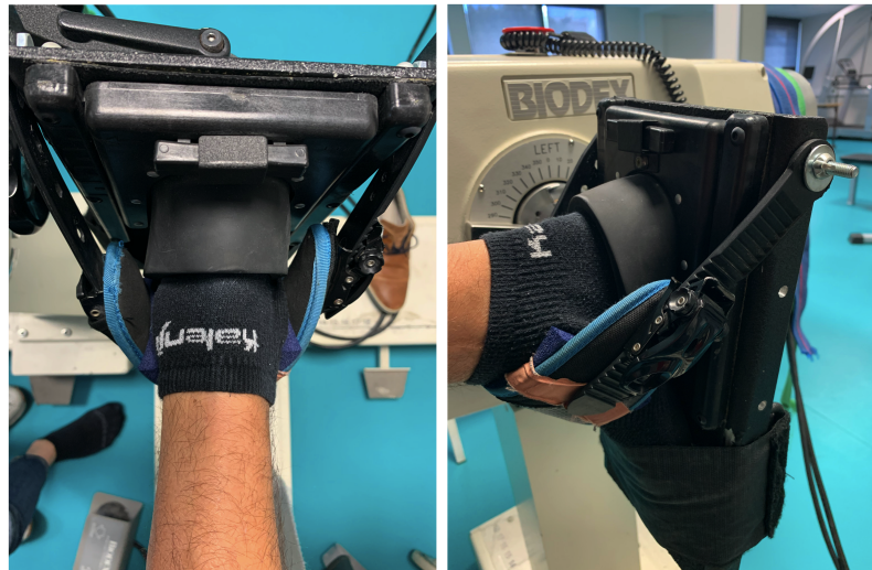
Figure 2: Modified ankle Biodex accessory. A snowboard binding was attached to the Biodex accessory to avoid any movement of the ankle and foot.
