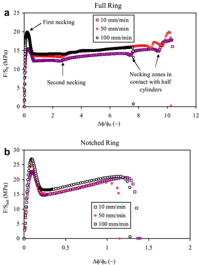
**Fig. 5.** Effect of crosshead speed on stress–strain complete curves. a) full ring: engineering stress ( $F/S_0$ ) versus engineering strain ( $\Delta\phi/\phi_0$ ) with  $S_0 = 12 \times 4.5 \times 2 = 108 \text{ mm}^2$  and  $\phi_0 = 31 \text{ mm}$ ; b) notched ring: net stress ( $F/S_{\text{net}}$ ) versus engineering strain ( $\Delta\phi/\phi_0$ ) with  $S_{\text{net}} = 6 \times 4.5 \times 2 = 54 \text{ mm}^2$  and  $\phi_0 = 31 \text{ mm}$ .
