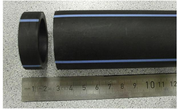
**Fig. 1.** HDPE material supply: full Nol ring specimen (slice of  $W = 12$  mm wide of the pipe). Nominal section is 4.5 mm  $\times$  12 mm = 54 mm<sup>2</sup> extracted from a pipe of 500 mm, thickness  $t = 4.5$  mm, internal diameter  $\phi_0 = 31$  mm.
