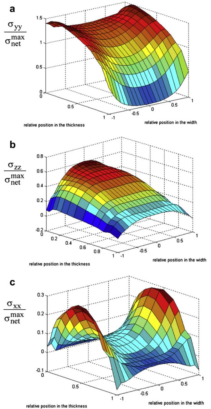
**Fig. 13.** Notched ring: 3D representation of the stresses distribution in the net section at maximum stress  $\sigma_{\text{net}}^{\text{max}} = 27$  MPa for 100 mm/mn crosshead speed. a) normalized hoop stress  $\sigma_{yy}/\sigma_{\text{net}}^{\text{max}}$ ; b) normalized longitudinal stress  $\sigma_{zz}/\sigma_{\text{net}}^{\text{max}}$ ; c) normalized radial stress  $\sigma_{xx}/\sigma_{\text{net}}^{\text{max}}$ .
