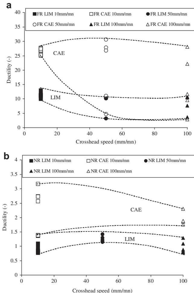
**Fig. 7.** Ductility a) Full ring; b) Notched ring.
