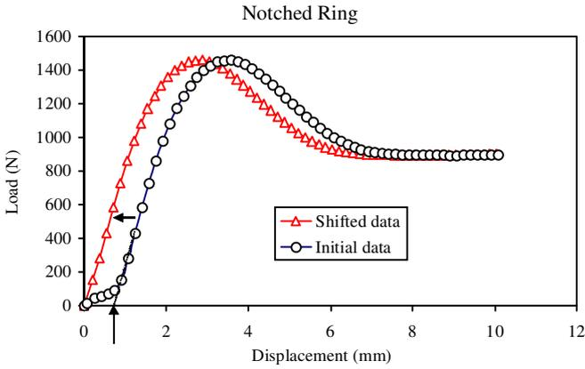
**Fig. 4.** Load versus applied displacement curve for notched ring at 100 mm/mn crosshead speed. Curve shifted to the left in order to avoid the effect of clearance reduction in the beginning of the test. This allows estimating the stiffness.
