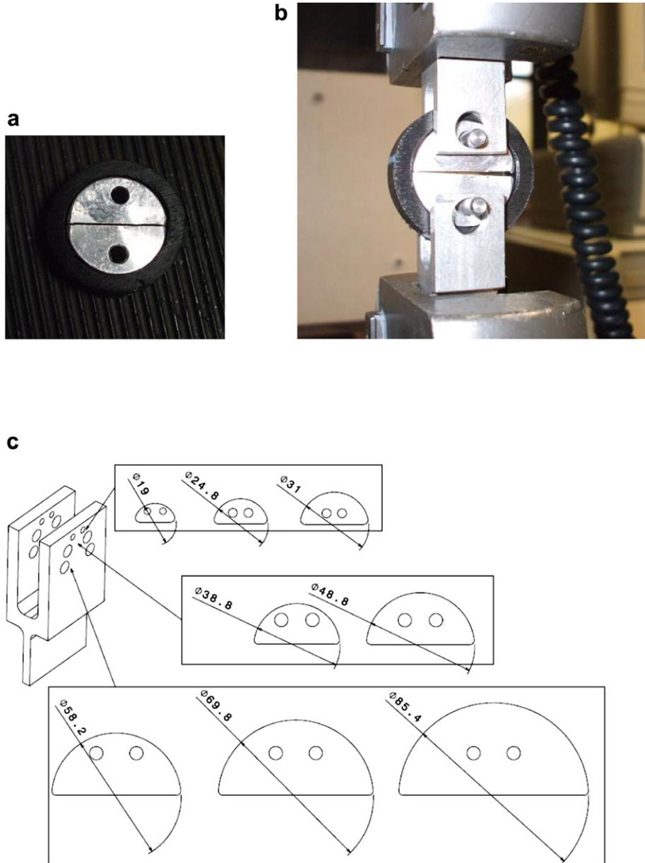
**Fig. 3.** Nol ring fixtures on the traction machine load-line: a) half disks with full ring; b) rotation of half disks, clearance in the right side of the ring is bigger than that of the left side; c) new fixture system for various ring diameters: fixation and smoothing of the sharp ends of half disks (*dimensions in mm*).
