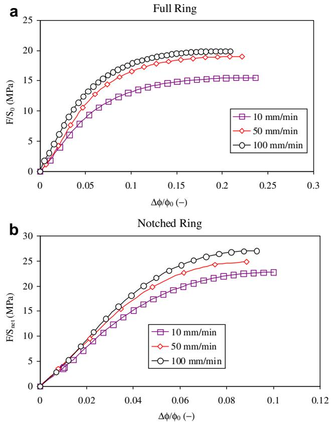
**Fig. 8.** Effect of crosshead speed on stress–strain curves up to maximum stress. a) full ring: engineering stress ( $F/S_0$ ) versus engineering strain ( $\Delta\phi/\phi_0$ ) with  $S_0 = 12 \times 4.5 \times 2 = 108 \text{ mm}^2$  and  $\phi_0 = 31 \text{ mm}$ ; b) notched ring: net stress ( $F/S_{net}$ ) versus engineering strain ( $\Delta\phi/\phi_0$ ) with  $S_{net} = 6 \times 4.5 \times 2 = 54 \text{ mm}^2$  and  $\phi_0 = 31 \text{ mm}$ .
