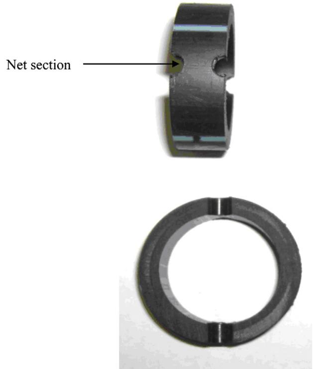
**Fig. 2.** Notched Nol ring specimen: notch radius  $\rho = 3$  mm obtained by "drilling". Net section is 4.5 mm  $\times$  6 mm = 27 mm<sup>2</sup>.
