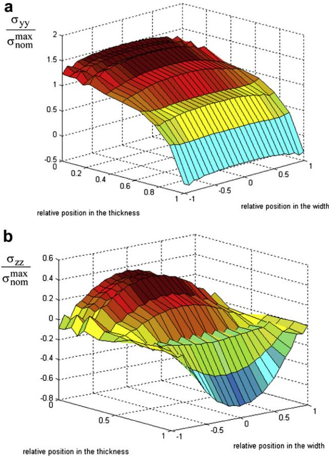
**Fig. 12.** Full ring: 3D representation of the stresses distribution in the cross section at maximum stress  $\sigma_{\text{nom}}^{\text{max}} = 20$  MPa for 100 mm/mn crosshead speed. a) normalized hoop stress  $\sigma_{yy}/\sigma_{\text{nom}}^{\text{max}}$ ; b) normalized longitudinal stress  $\sigma_{zz}/\sigma_{\text{nom}}^{\text{max}}$ .
