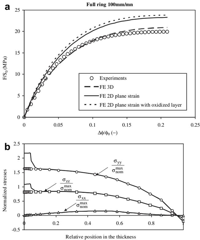
**Fig. 14.** Curves comparing full ring with/without 200  $\mu\text{m}$  layer of oxidized material, at maximum stress  $\sigma_{\text{nom}}^{\text{max}} = 20 \text{ MPa}$  for 100 mm/mn crosshead speed. a) stress–strain curves; b) normalized stresses.
