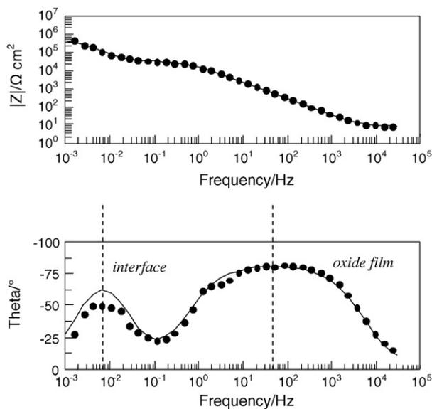
**Fig. 4.** Local impedance diagram (Bode representation) on pure aluminium. Experiments were conducted after immersion of aluminium in 0.1 M NaCl at the OCP value for 25 min using 50  $\mu\text{m}$  diameter capillaries. The line represents the model data corresponding to the equivalent circuit in Fig. 3(c).
