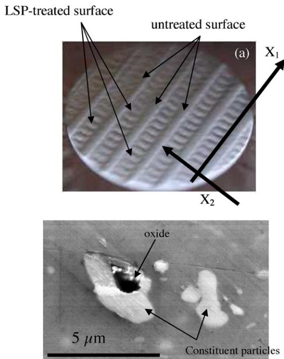
**Fig. 1.** (a) Optical image of the sample after LSP treatment.  $X_1$ - and  $X_2$ -axes used for stress measurements are indicated. (b) FE-SEM/EDS image of constituent particles in AA2050-T8 after mechanical polishing.
