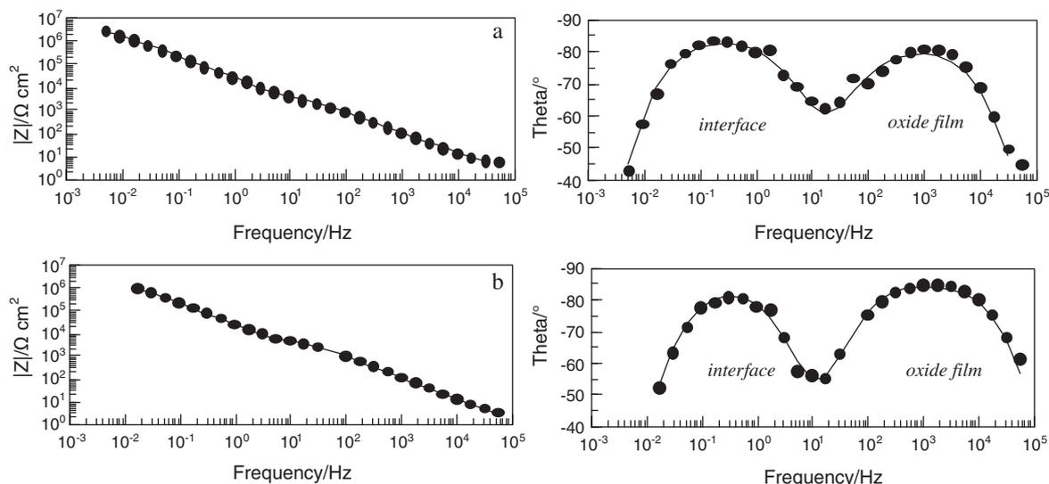
**Fig. 6.** Local electrochemical impedance diagrams (Bode representation) obtained on the untreated surface. Investigated sites contain the (a) matrix and (b) the matrix with constituent particles. Experiments were conducted after immersion of AA2050-T8 in 0.1 M NaCl at the OCP value for 25 min using 50  $\mu\text{m}$  diameter capillaries. The lines represent the model data corresponding to the equivalent circuit in Fig. 3(c).
