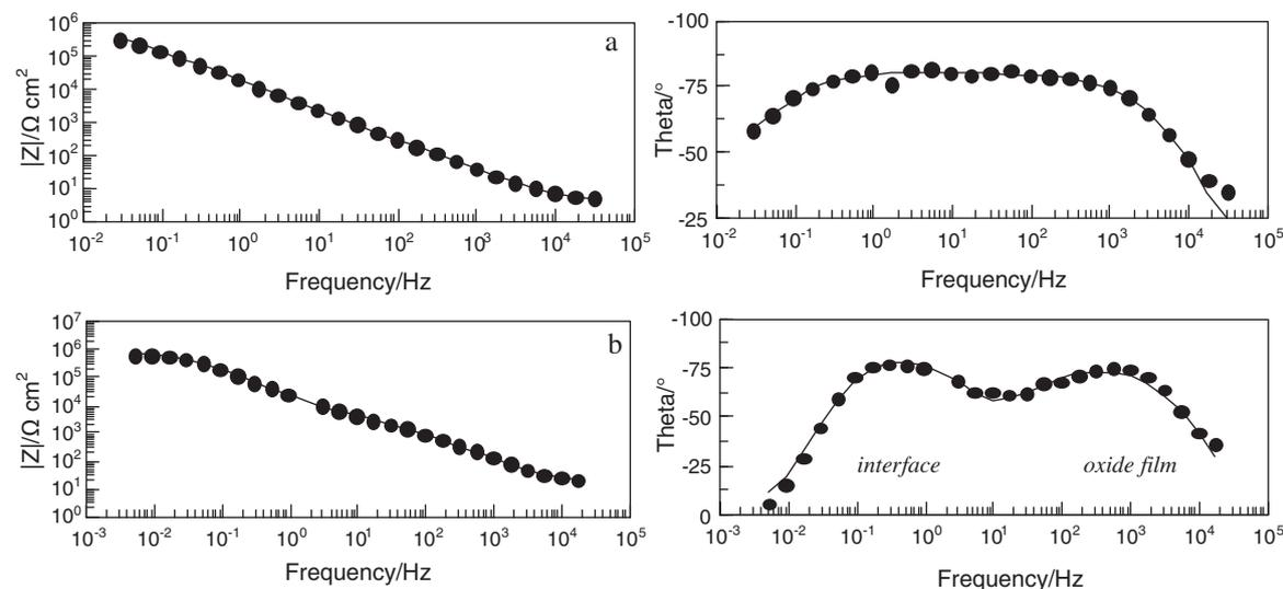
**Fig. 7.** Local electrochemical impedance diagrams (Bode representation) obtained on the LSP treated surface. Investigated sites contain the (a) matrix and (b) the matrix with constituent particles. Experiments were conducted after immersion of AA2050-T8 in 0.1 M NaCl at the OCP value for 25 min using 50  $\mu\text{m}$  diameter capillaries. Lines represent the model data corresponding to the equivalent circuit in Fig. 3(c).
