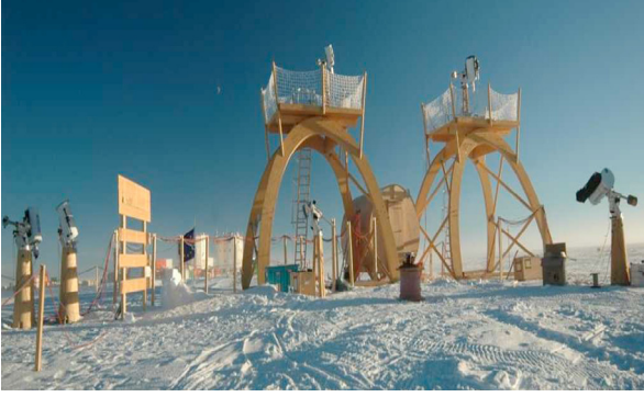
Fig. 4. Site-testing instrumentation at Dome C during winter 2006. The GSM instrument ( left ) is protected from the prevailing wind by a wood screen.
