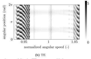
Figure 18. Evolution of the wear profile with the angular speed for the HP compressor blade.
