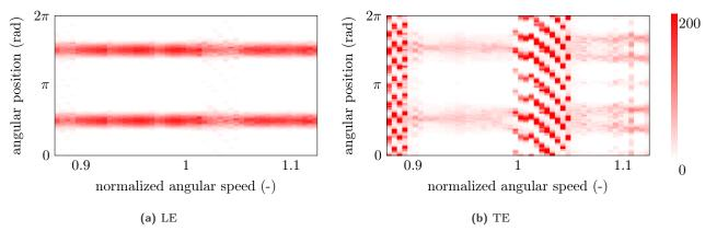
Figure 26. Evolution of the temperature profile with the angular speed for the LP compressor blade.
