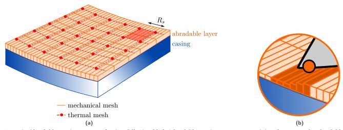
**Figure 2.** Abradable coating wear mechanism following blade/abradable coating contact event (**a**) and zoom on the abradable layer's wear (**b**).
