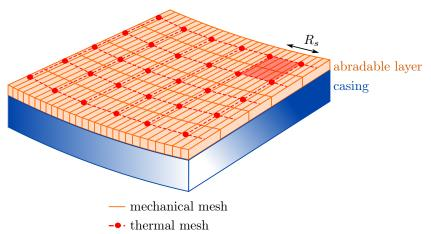
Figure 3. Superimposed mechanical and thermal meshes.
