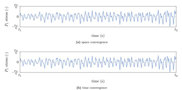
Figure 7. Time evolution of blade stresses (a) with  $R_s$ :  $R_s = 80$  ((—)),  $R_s = 100$  ((—)),  $R_s = 200$  ((—)),  $R_s = 200$  ((—)),  $R_t = 1000$  ((—)),  $R_t = 1000$  ((—)).
