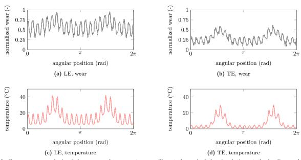
Figure 6. Convergence analysis of the wear and temperature profiles at the end of the simulation at the leading and trailing edge with  $R_t$ :  $R_t = 1$  ((—)/(—)),  $R_t = 500$  ((—)/(—)),  $R_t = 5000$  ((—)/(—)).
