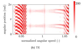
Figure 19. Evolution of the temperature profile with the angular speed for the HP compressor blade.
