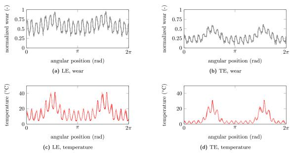
Figure 5. Convergence analysis of the wear and temperature profiles at the end of the simulation at the leading and trailing edge with the number of thermal abradable coating elements  $n_{ab,th}$ :  $n_{ab,th} = 80$  or  $R_s = 250$  ((—)/(—)),  $n_{ab,th} = 100$  or  $R_s = 200$  ((—)/(—)),  $n_{ab,th} = 200$  or  $R_s = 100$  ((—)/(—)),  $n_{ab,th} = 250$  or  $n_{ab,th} = 250$
