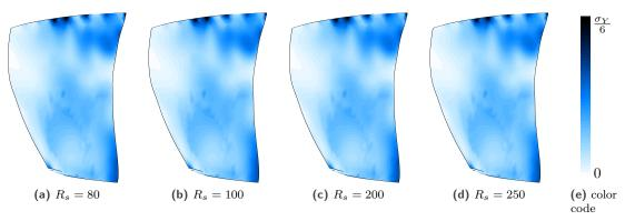
Figure 8. Blade stress fields for different  $R_s$  values.
