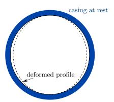
Figure 1. 2-lobe casing deformation.
