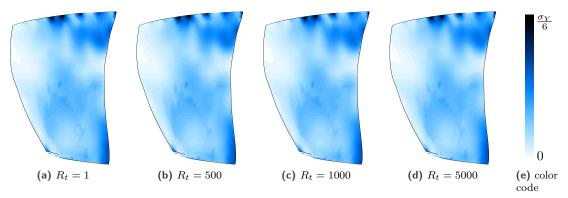
Figure 9. Blade stress fields for different  $R_t$  values.
