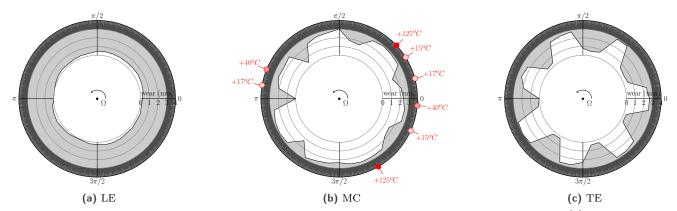
Figure 15. Experimental wear and temperature profiles for the LP compressor test case [2].
