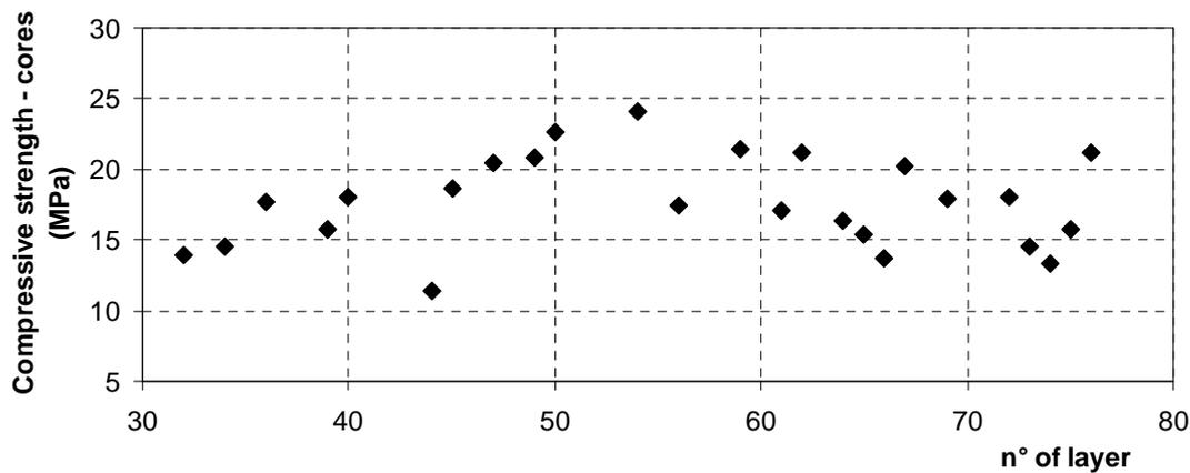
**Figure 2.** Example of Compressive Strength Values Measured at End of Construction of an RCC Dam on Drill Core
