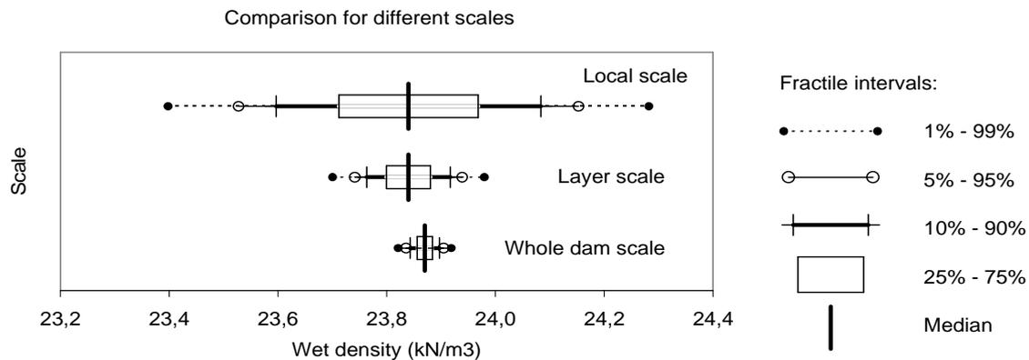
**Figure 10.** Scatter in Densities vs Spatial Scale – Example for RCC layer 31
