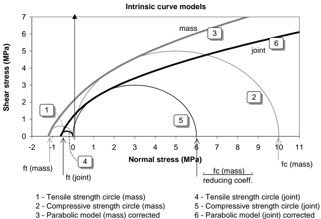
**Figure 7.** Parabolic Model for RCC Mass and Construction Joint Intrinsic Curve
