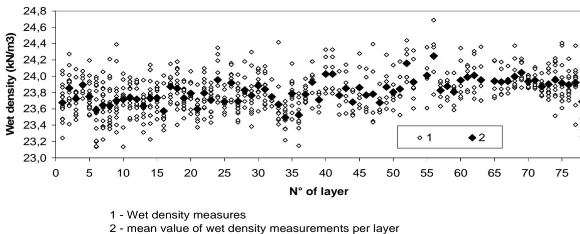
**Figure 1.** Typical RCC Densities Measured in Compaction Control Tests on an RCC Dam, for Each Layer
