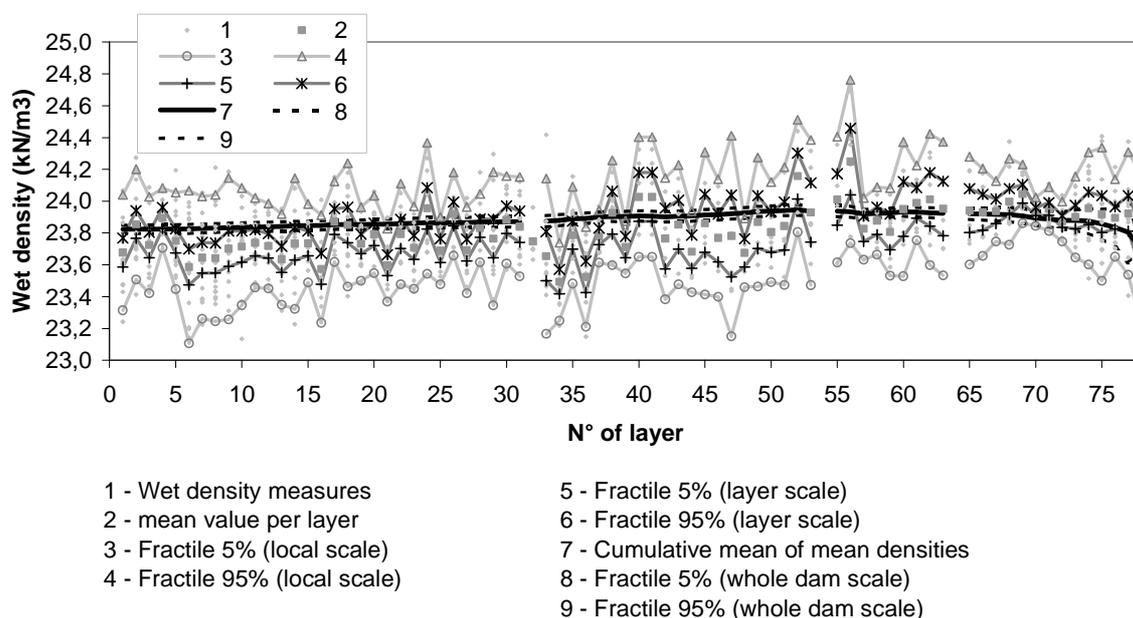
**Figure 9.** Density Modelling at Local, Layer and Whole Dam Scales
