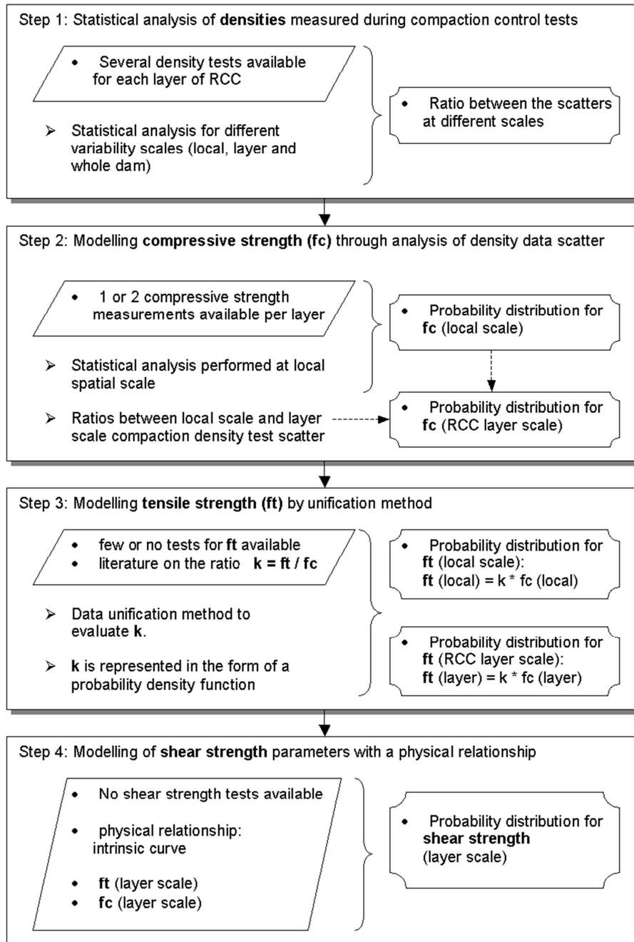
**Figure 4.** General Procedure Proposed for Modelling Shear Strengths
