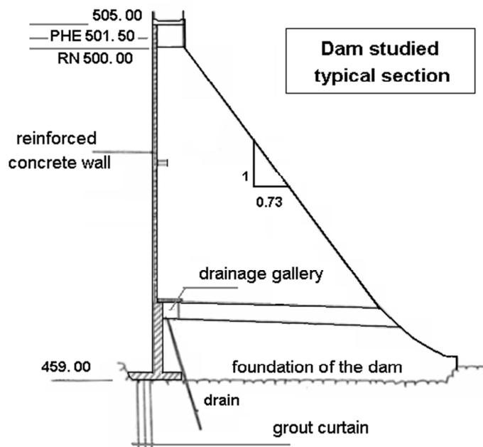
**Figure 8.** Typical Section through RCC Dam
