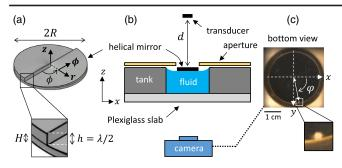
FIG. 1. Acoustic radiation torque experiment. (a) Designed helical mirror, here with  $\ell = 2$ , with  $(\mathbf{r}, \boldsymbol{\phi}, \mathbf{z})$  the unit vectors of the cylindrical basis. (b) Sketch of the setup, where the camera is used to record the rotational dynamics of the helical mirror from its flat side. (c) *In situ* bottom view of a helical mirror, where the printed marker is on the back side of the mirror used to monitor its angular dynamics  $\varphi(t)$ .
