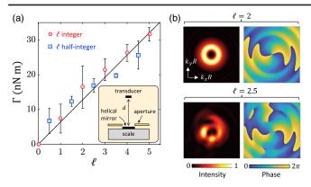
FIG. 5. (a) Acoustic torque as a function of its topological charge. Markers: experimental data. Solid line: linear fit. Inset refers to radiation force balance measurement.(b) Calculated far-field normalized intensity and phase distribution of the wave reflected off the helical mirror for  $\ell = 2$  and 2.5. Panels refers to the range  $-5 \le (k_x R, k_y R) \le 5$ .
