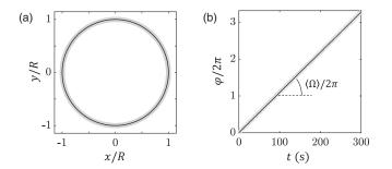
FIG. 3. (a) Typical trajectory, in the (x, y) plane, of the marker at the backside of the spinning helical mirror over ~3 full turns. (b) Experimental dynamics of the azimuthal angular coordinate of the marker  $\varphi$ , which is evaluated from the trajectory shown in panel (a), taking  $\varphi = 0$  at t = 0. Data refer to an  $\ell = 5$  helical mirror. Thick gray curve: experimental data. Thin dark circle: best circular (a) and linear (b) fit.
