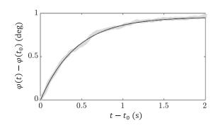
FIG. 4. Typical relaxation dynamics of the angular position of the helical mirror, where  $t = t_0$  refers to the time at which the acoustic source is turned off. Thick gray curve: experimental data. Thin dark curve: fit giving access to the ratio C/J. Data refer to an  $\ell = 5$  helical mirror.
