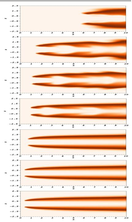
**Figure 1.** Snapshots at t = 200 of jet flames obtained by seven DNSs with:  $Da = 1 \times 10^5$ ,  $1.5 \times 10^5$ ,  $2 \times 10^5$ ,  $3 \times 10^5$ ,  $4 \times 10^5$ ,  $5 \times 10^5$ ,  $6 \times 10^5$  (top to bottom). Contours of non-dimensional temperature in a y = 0 plane. Scales are from white  $(1 \times 0^{-2})$  to red (0.98).
