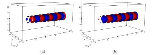
**Figure 12.** Isosurfaces of the non-dimensional temperature T (a) and of the mixture fraction Z for the real component of mode B at  $Da = 6.0 \times 10^5$ . Negative (blue) and positive (red) surfaces are shown.
