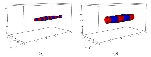
**Figure 6.** Isosurfaces of the non-dimensional temperature T (a) and of the mixture fraction Z (b) for the real component of the most unstable weak-flame global mode at  $Da = 1.5 \times 10^5$ . Negative (blue) and positive (red) surfaces are shown.
