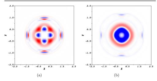
**Figure 11.** Non-dimensional temperature distribution in the cross sections at x = 4.5 (a) and x = 8.0 (b) for the real component of mode A at  $Da = 6.0 \times 10^5$ . Negative (blue) and positive (red) contours are shown.
