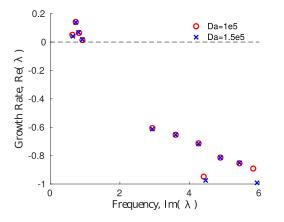
**Figure 5.** The least-stable part of the global eigenvalue spectra for the weak flame cases at  $Da = 10^5$  (circles) and  $Da = 1.5 \times 10^5$  (crosses).
