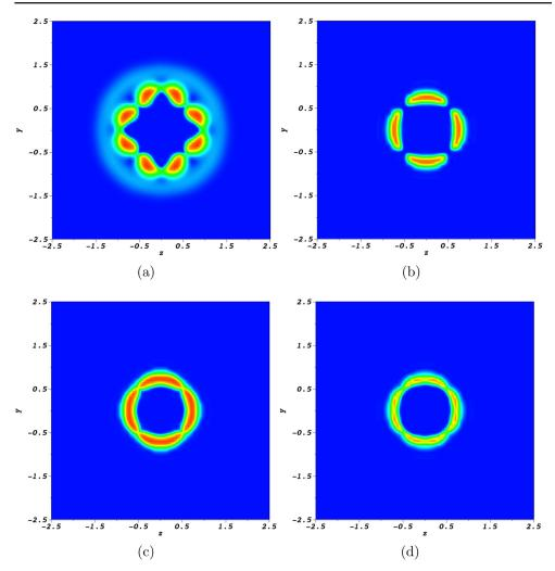
**Figure 2.** Non-dimensional temperature contours in a cross section showing the computed cellular structures: (a)  $Da = 10^5$ , x = 4; (b)  $Da = 1.5 \times 10^5$ , x = 1; (c)  $Da = 2 \times 10^5$ , x = 1.15; (d)  $Da = 3 \times 10^5$ , x = 1.1. Scales are from blue (low) to red (high).
