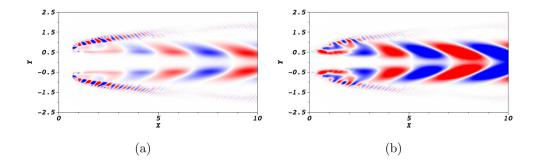
**Figure 10.** Contours of the non-dimensional temperature T (a) and of the mixture fraction Z (b) in a longitudinal plane for the real component of mode A at  $Da = 6.0 \times 10^5$ . Negative (blue) and positive (red) contours are shown.
