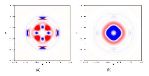
**Figure A2.** Non-dimensional temperature distributions in the cross sections at x = 4.5 (a) and x = 8.0 (b) for the real component of mode A obtained for  $Da = 6 \times 10^5$ .
