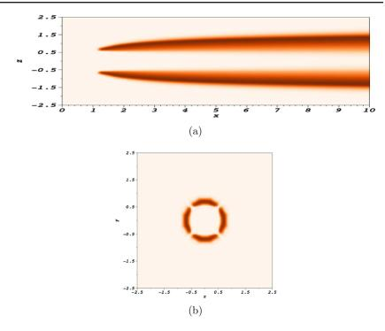
**Figure 3.** Base flow of cellular jet flame: non-dimensional temperature field in the longitudinal section (a) and in the crosswise section at x = 1.3 (b) for  $Da = 2.0 \times 10^5$ . Same temperature scale as figure 1.
