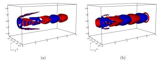
**Figure 9.** Isosurfaces of the non-dimensional temperature *T* (a) and of the mixture fraction *Z* (b) for the real component of mode A at  $Da = 6.0 \times 10^5$ . Negative (blue) and positive (red) surfaces are shown.
