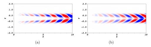
**Figure 13.** Contours of the non-dimensional temperature T (a) and of the mixture fraction Z (b) for the real component of mode B at  $Da = 6.0 \times 10^5$ . Negative (blue) and positive (red) contours are shown.
