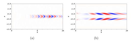
**Figure 7.** Contours of the non-dimensional temperature T (a) and of the mixture fraction Z (b) in a longitudinal plane for the real component of the most unstable weak-flame global mode at  $Da = 1.5 \times 10^5$ . Negative (blue) and positive (red) contours are shown.
