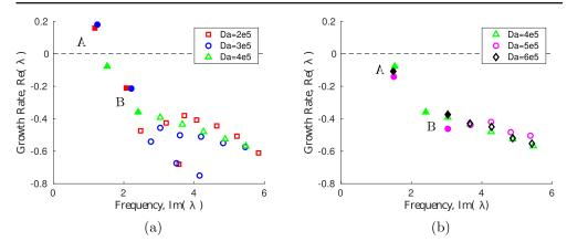
**Figure 8.** Global eigenvalue spectra for cellular flames at (a)  $Da = 2 \times 10^5$ ,  $Da = 3 \times 10^5$  and  $Da = 4 \times 10^5$ ; (b)  $Da = 4 \times 10^5$ ,  $Da = 5 \times 10^5$  and  $Da = 6 \times 10^5$ . Filled symbols represent modes A and B.
