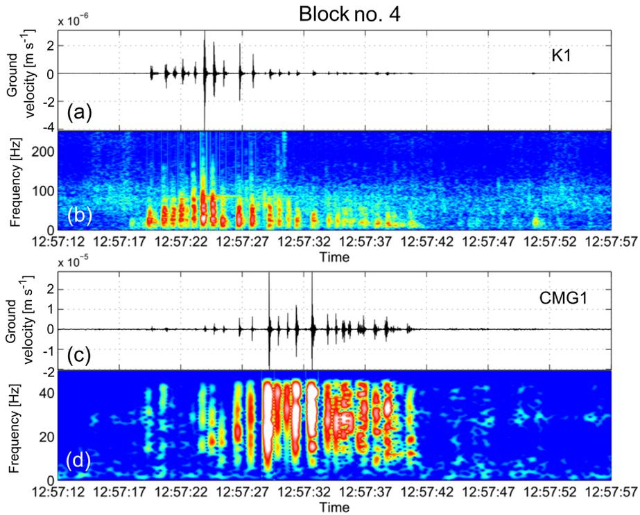
**Figure 2.** (a) Signal recorded at the short-period station located on the upper part of the slope and (b) corresponding spectrogram, generated by block number 4 (mass of 209 kg). (c) Signal recorded at the broadband station located on the lower part of the slope and (d) corresponding spectrogram, generated by block 4.
