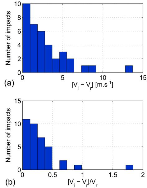
**Figure 5.** (a) Histogram showing the distribution of the difference between the velocity before impact  $V_i$  inferred using Eqs. (7) and (8) and the velocity  $V_r$  estimated from the video cameras. (b) Same as (a) but normalized by the value of the velocity  $V_r$  estimated via the video cameras.
