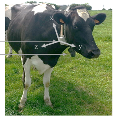
Fig. 2. RF-Track 3D accelerometer and GPS sensor fixed on the collar on the cow. The three coordinate axes of the accelerometer sensor are displayed.
