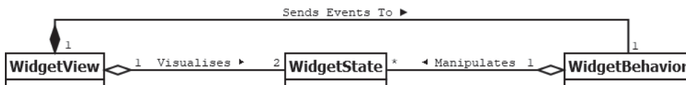
Fig. 11. Each WidgetView is capable of visualizing two instances of WidgetState simultaneously: the current and the future state.
