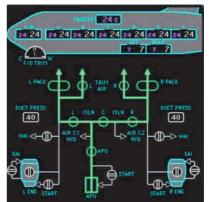
Figure 5. The B777 AIR synoptic page present both BLEED and AIR COND information
