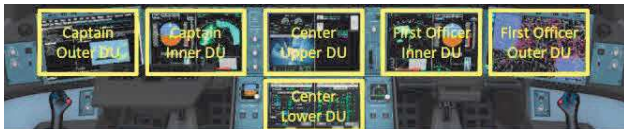
Figure 1. Display Units layout on the Airbus A350 Main Instrument Panel.
