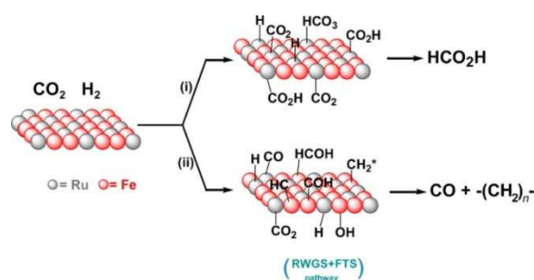
Figure 22. Representation of mechanistic route for the chemoselective hydrogenation of CO 2 by RuFe NPs in ILs. Reprinted with permission from ref 256 . Copyright 2018 American Chemical Society.
