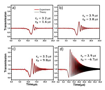
Fig. 2. Transient responses of the probed cavity mode for various laser pump powers. From a) to d) the resonator-coupling regime shifts with increasing pump power from under coupling ( $P_{in}=13.8~\text{mW}$ ), critical coupling ( $P_{in}=39.1~\text{mW}$ ), over coupling ( $P_{in}=41.7~\text{mW}$ ) and selective amplification regime ( $P_{in}=58.5~\text{mW}$ ). The sweeping speed extracted from the theoretical fit gives  $\tilde{V}_s=2.8MHz/\mu s$
