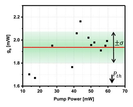
Fig. 3. Brillouin gain coefficient extracted from the CRDM signal for various input pump power. The mean value is equal to  $g_B = 1.94 \times 10^{-11} \pm 1.5 \times 10^{-12} m/W$ . This measure of  $g_B$  value is compared to other works in Tab. 2
