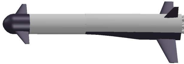
Figure 2: Glide-back configuration with the components of the reusability kit (in black)
