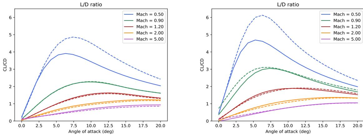
Figure 10: Lift over Drag ratio between NACA (dash line) and double-wedge (solid line) airfoil profiles, as a function of Mach number and angle of attack. Two configurations are evaluated: wingspan equivalent to three times the stage diameter (left), wingspan equivalent to five times the stage diameter (right).
