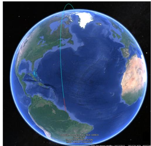
(b) Illustration of the ascent trajectory for SSO orbit
