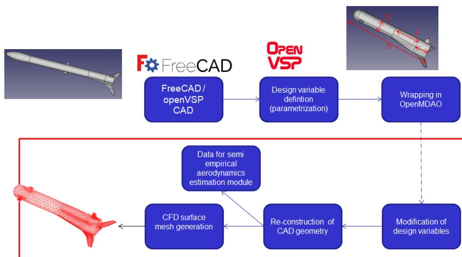
Figure 3: Illustration of geometry discipline
