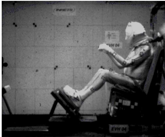
Figure 1. Rigid seat for the HUMOS sled tests.
