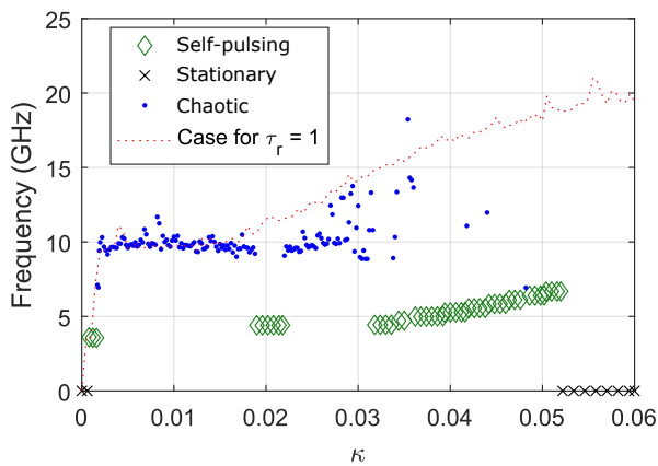
Figure 6: Theoretical variation of chaos-bandwidth (for chaotic state) and oscillation frequency (for self-pulsing states) of a laser with filtered PCF, versus the feedback rate. The red dotted line is the chaos bandwidth of an instantaneous PCF.
