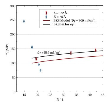
Figure 8: Critical resolved shear stress  $\tau_c$  for an edge dislocation to pass  $Mg_{17}Al_{12}$  precipitates with a constant spacing L and varying diameter D, as well as constant D and varying L plotted against the harmonic mean,  $\bar{D}$ . Atomistic simulations (data points), BKS model using  $\delta \gamma = \gamma_{\text{interface}}$  (red line) and with fitted  $\delta \gamma$  (black line).
