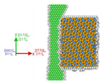
**Figure S6:** Top view of a cut just above the dislocation glide plane showing an edge dislocation in front of the precipitate upon energy minimization at  $\tau = 0$  MPa for the *default setup*. The defect atoms in the Mg matrix are colored as green (fcc) and white (other), while the atoms in the precipitate are colored based on atomic species – Mg (orange), Al (blue). The hcp coordinated matrix atoms are not shown.
