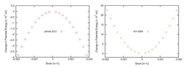
Figure S1: Change in potential energy of an Mg<sub>17</sub>Al<sub>12</sub> sample with applied shear strain
