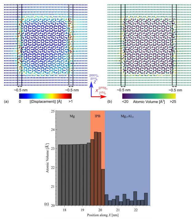
**Figure S3:** Side view showing the width of the Mg-Mg<sub>17</sub>Al<sub>12</sub> interface for a relaxed precipitate in the matrix following the Burgers orientation relationship computed using (a) Displacement magnitude with respect to the perfect lattice positions, and (b) atomic volume. (c) Histogram of atomic volume for the region around the left interface with a binning width of 2Å showing an increased excess volume.
