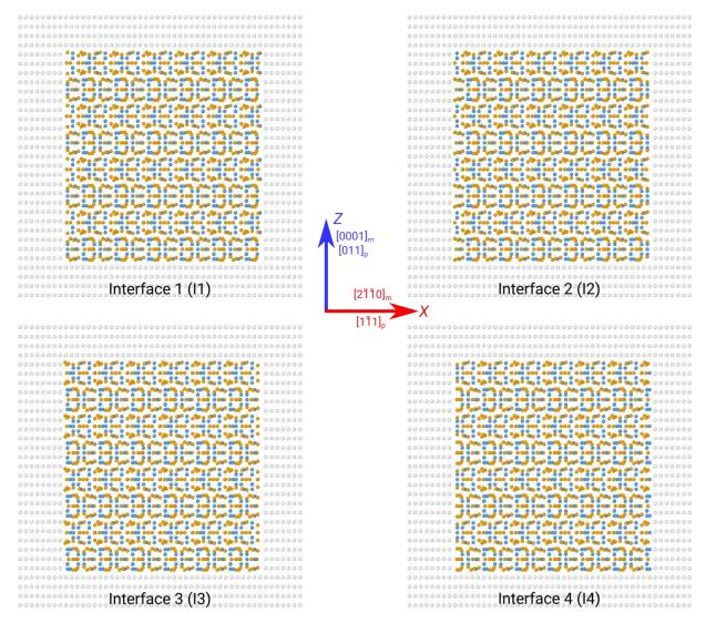
**Figure S2:** Different interface terminations of the  $Mg_{17}Al_{12}$  precipitate (orange: Mg, blue Al) embedded in the Mg matrix (grey atoms) studied in the present work. The interface number correspond to those presented in the Fig. 1 of the main manuscript.
