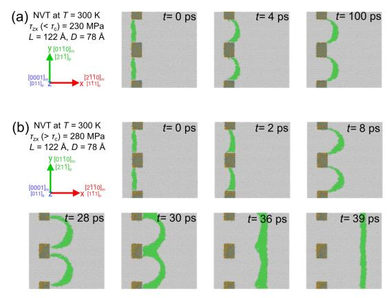
**Figure S7:** Infinite basal edge dislocation interacting with a periodic array of  $Mg_{17}Al_{12}$  precipitates using molecular dynamics NVT simulation at T = 300 K with an applied shear stress (a) smaller, and (b) larger than the critical resolved shear stress (L = 122Å, D = 78Å). The Mg atoms in the matrix are colored grey and the defect fcc atoms in the Mg matrix green, while the atoms in the precipitate are colored based on atomic species – Mg (orange), Al (blue).
