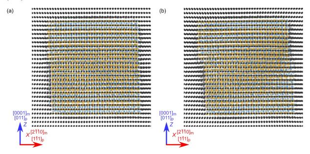
**Figure S5:** Side view showing the relaxed local disordered region at the Mg-Mg<sub>17</sub>Al<sub>12</sub> IPB for the *default setup* (a) with one absorbed dislocation at  $\tau = 240$  MPa, (b) with two absorbed dislocations after passage of the first dislocation at  $\tau = 250$  MPa. The matrix atoms are dark grey, while the atoms in the precipitate are colored based on atomic species – Mg (orange), Al (blue).
