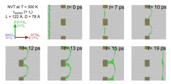
**Figure S8:** Infinite 30° mixed dislocation interacting with a periodic array of  $Mg_{17}Al_{12}$  precipitates using molecular dynamics NVT simulation at T=300~K with an applied shear stress larger than the critical resolved shear stress ( $L=122\text{\AA}$ ,  $D=78\text{\AA}$ ). The Mg atoms in the matrix are colored grey and the defect fcc atoms in the Mg matrix green, while the atoms in the precipitate are colored based on atomic species – Mg (orange), Al (blue).
