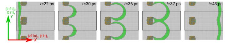
Figure 7: Snapshots of a second infinite straight basal edge dislocation interacting with a periodic array of Mg<sub>17</sub>Al<sub>12</sub> precipitates for the default setup (NVE at  $T_0 = 0 \,\mathrm{K}$ ,  $\tau_{\mathrm{zx}} = 270 \,\mathrm{MPa}$ ). See fig. 1 for the color coding.
