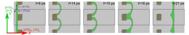
Figure 5: Snapshots of an infinite straight basal 30° dislocation interacting with a periodic array of  $Mg_{17}Al_{12}$  precipitates, as simulated by molecular dynamics (NVE at  $T_0 = 0 \, \text{K}$ ,  $\tau_{\text{applied}} = 280 \, \text{MPa}$ ). Color coding, see Fig. 1.
