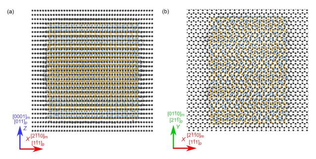
**Figure S4:** (a) Side view and (b) top view showing the local disordered region at the Mg-Mg<sub>17</sub>Al<sub>12</sub> IPB for a relaxed precipitate in the matrix following the Burgers orientation relationship. The matrix atoms are dark grey, while the atoms in the precipitate are colored based on atomic species - Mg (orange), Al (blue).
