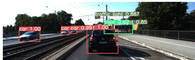
Figure 3. Result of YOLOv3 [2] (Returns the position, class and score of trust of each detected object).
