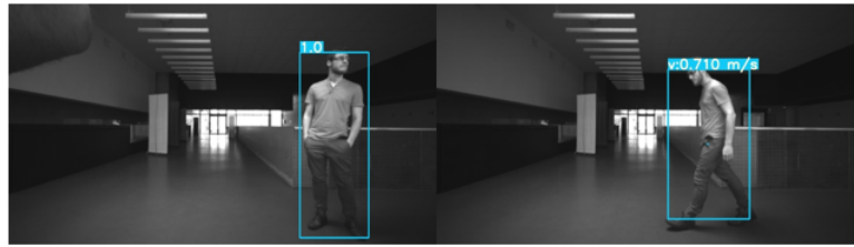
Figure 10. Result of the tracking approach over an indoor scene using the stereo images provided by the Intel RealSense D435 sensor. The left frame is acquired at instant t = 1 and the right one at the instant t + 3 . At t = 1 , we assign an ID to each detected object. Then, at t + 3 , the tracklet is validated and we display the estimated speed.
