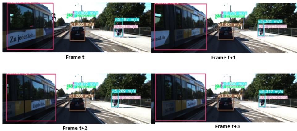
Figure 11. Tracking results in the road environment.
