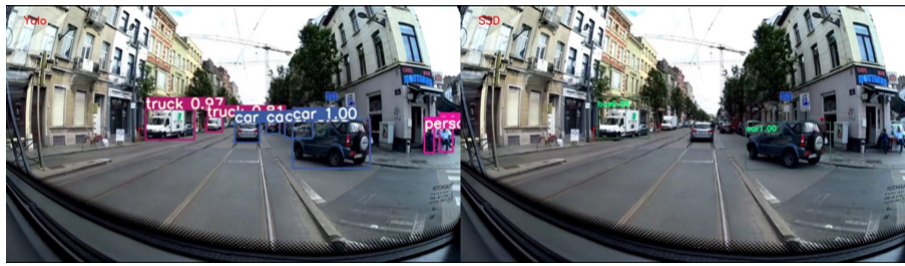
Figure 4. Performance comparison between YOLOv3 (left) and SSD (right) detectors.
