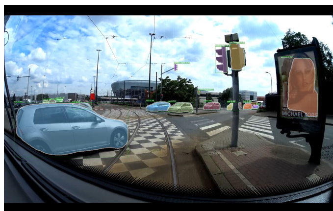
Figure 2. Mask-RCNN results (returns the mask of each detected object with their class and their confidence score).
