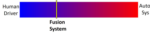
Fig. 1. The presented methodology creates a continuous control authority scale between the human driver and AutoSys. An example of control authority division using fusion system.
