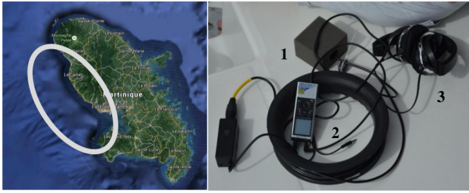
Figure 1. Presentation of the study area and material (1: Hydrophone (in its protection), 2: recorder and 3: headphone).
