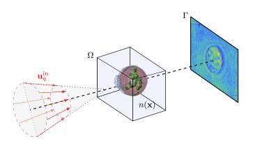
**Fig. 1.** Principle of optical diffraction tomography. The wave vectors  $\{\mathbf{k}_q^{\text{in}}\}_{q=1}^Q \in \mathbb{R}^3$  of the Q incident plane waves  $\{u_q^{\text{in}}\}_{q=1}^Q$  are limited to a cone around the optical axis.
