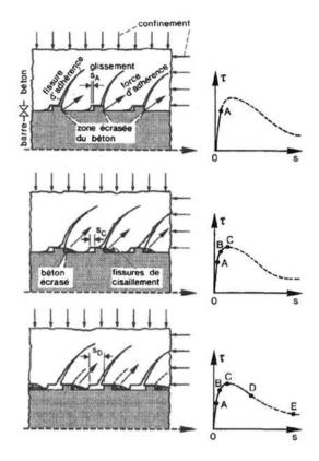
Figure 5. Adhesion mechanism and diagram from the full bond-sliding relationship according to Eligehausen et al. [27].
