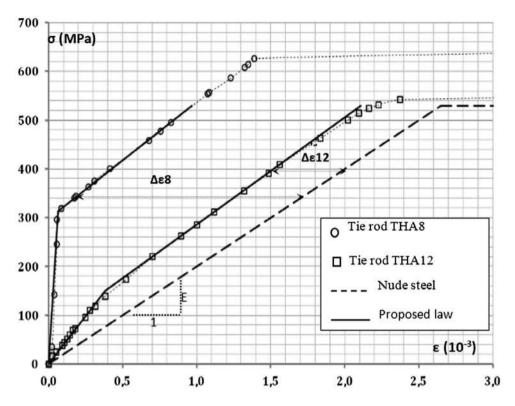
Figure 12. Diagrams  $\sigma - \varepsilon_t$  of tie-rodsTHA8 and THA12.
