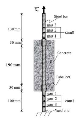
Figure 11. Tie-rods in tension.
