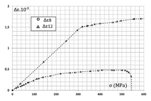
Figure 13. Diagrams  $\Delta \epsilon_t - \sigma$  of tie-rodsTHA8 and THA12.
