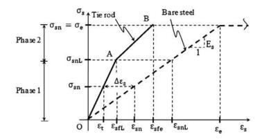
**Figure 3.** Diagram type  $\sigma - \varepsilon$  of the short tie.
