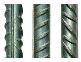
Figure 6. High adhesion steel used.
