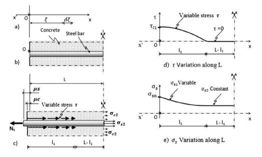
Figure 4. Slipping between steel and concrete and stresses generated under N, in the tie.
