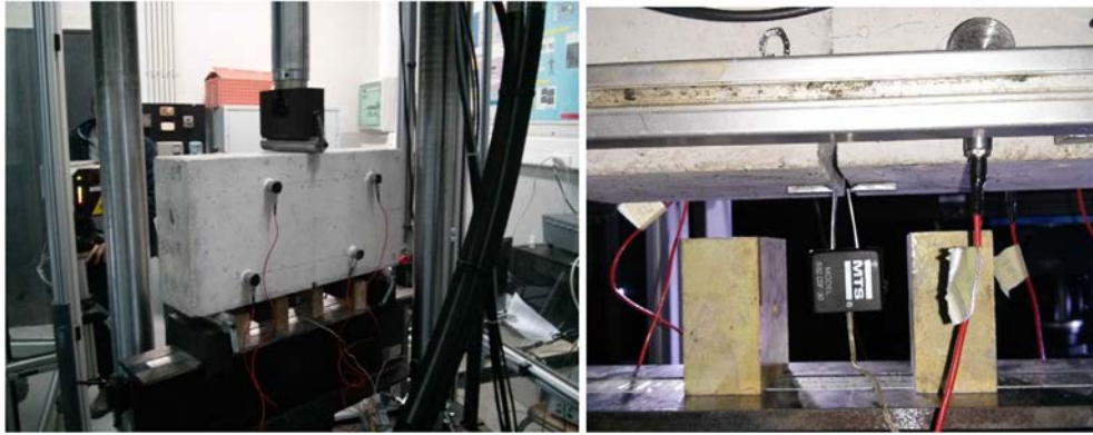
Fig. 1. Three point bending test on concrete beam (a). MTS CMOD device (b).
