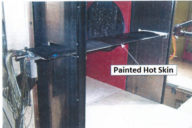
Fig. 11 ONERAD airfoil experimental setup with hot skin in ONERA F2 wind tunnel
