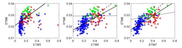
Figure 2: relations between reflectances in ETM6 and ETM3 (left), ETM5 (centre) and ETM7 (right). V: LSL data, V: LSL dry data, o: ASTER data; Black line; regression over the whole dataset; dashed line: regression over LSL; dotted line: regression over the dry soils data.
