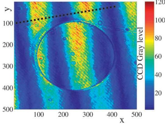
Figure 3. Image of the fringe pattern showing the phase-shift through the transparent phase object. The dashed line in the upper left side represents the  $\Delta$  axis perpendicular to the fringes chosen by the operator for *in situ* calibration and space fringe measurement, as is done in Figure 2(b). The vertical bar represents the CCD gray level. (The color version of this figure is included in the online version of the journal.)
