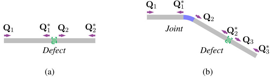
Figure 3: Schematics of one waveguide with a defect (a), and of one waveguide assembly with a curved joint and a defect (b).
