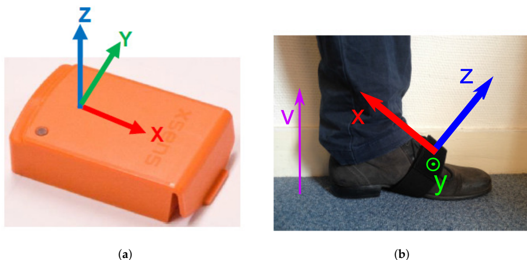
Figure 1. Presentation of the XSens™ sensor. (a) XSens™ sensor; (b) Definition of the axis for the XSens™ sensor located at the left foot.
