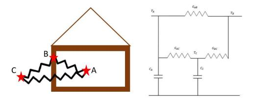
Figure 3: Two-node (or R3C2 model) thermal system representation of the building
