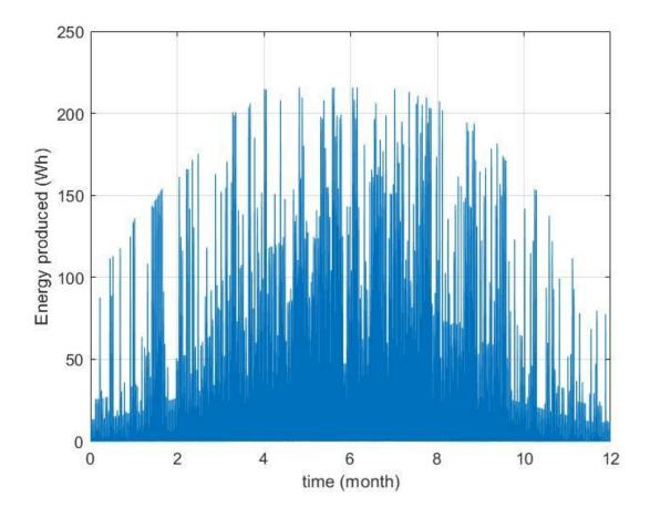
Figure 2 : Solar production throughout the year for the case of the Montreal area in optimal position
