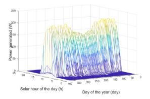
Figure 11: Solar production for one array in the Montreal area tilted towards south at: 70° (right) and 30° (left)
