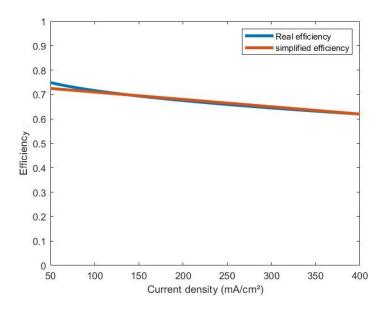
Figure 4: Real and simplified efficiency of the electrolyzer
