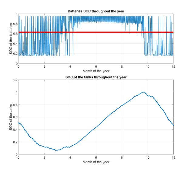
Figure 8: SoC of the batteries and the tanks throughout the year
