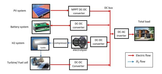
Figure 1: Schematic diagram of the stand-alone hybrid system
