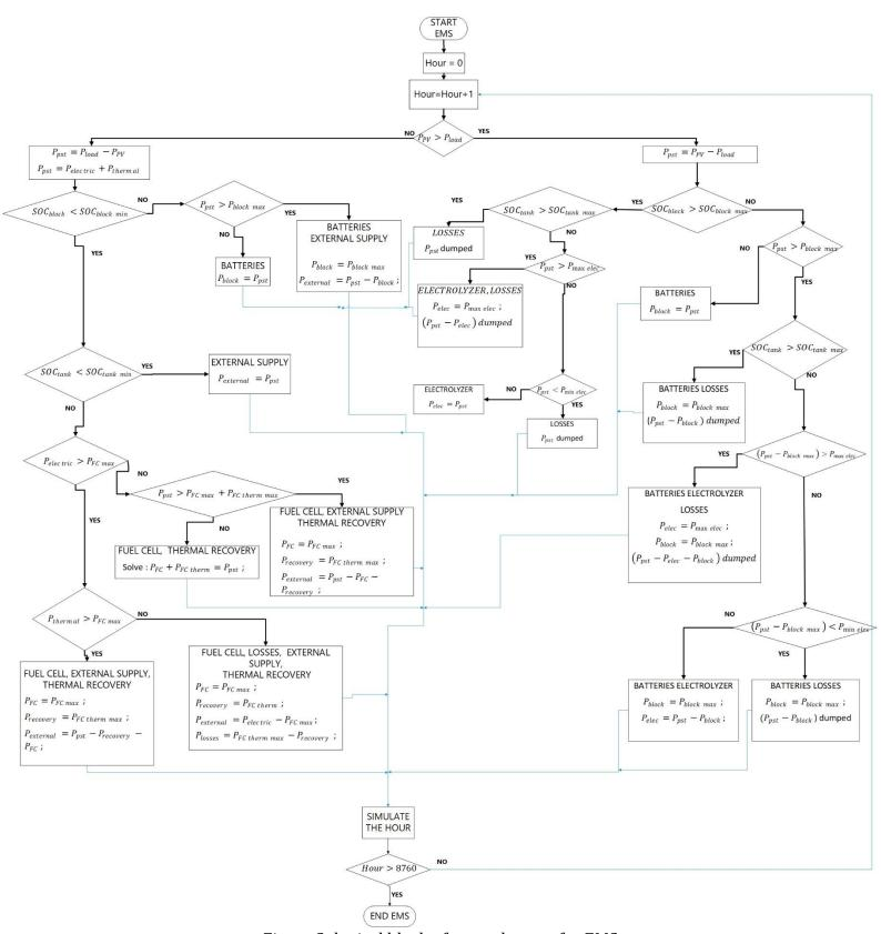
Figure 2: logical block of control states for EMS
