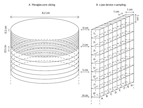
**Figure 2.** Sediment sampling methodology for living foraminiferal analyses. (a) Usual 1-D hand coring and layer slicing. (b) Sediment plate sampling with the second jaw of the "jaw device" (Fig. 1) and representation of the sediment cubic slicing.
