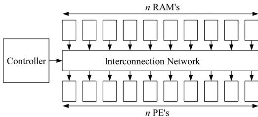
Fig. 1. Parallel structure of a QC-LDPC decoder.
