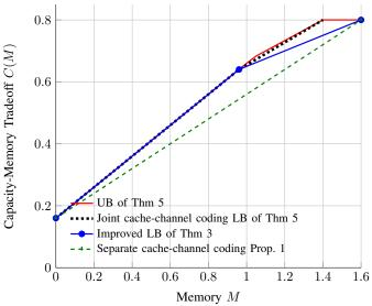
Fig. 7: Bounds on the capacity-memory tradeoff for  $K_w = 1$ ,  $K_s = 1$ , D = 2,  $\delta_w = 0.8$ ,  $\delta_s = 0.2$ .
