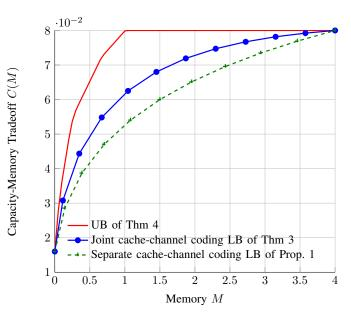
Fig. 5: Bounds on the capacity-memory tradeoff C(M) for  $K_{\rm w} = K_{\rm s} = 10, D = 50, \delta_{\rm w} = 0.8, \delta_{\rm s} = 0.2.$
