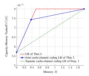
Fig. 6: Bounds on the capacity-memory tradeoff for  $K_w = 1$ ,  $K_s = 10$ , D = 22,  $\delta_w = 0.8$ ,  $\delta_s = 0.2$ .
