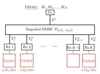
Fig. 4: Degraded K-user BC  $P_{Y_1Y_2\cdots Y_K|X}$  where each receiver  $k \in \mathcal{K}$  has cache memory of size  $nM_k$  bits.
