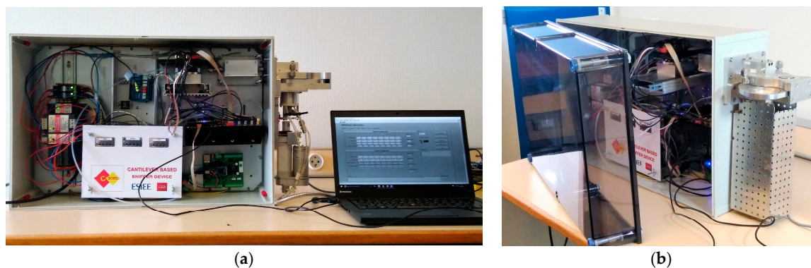
Figure 4. Pictures of the Sniffer System (a) A global view of the system: opened box containing the integrated system, the thermodesorber and a computer for human-machine interface (b) Another view of the system where we can see more details of the thermodesorber.
