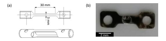
Figure 1 : (a) geometry of a two-leg macro-tensile specimen, (b) geometry of a micro-tensile specimen.
