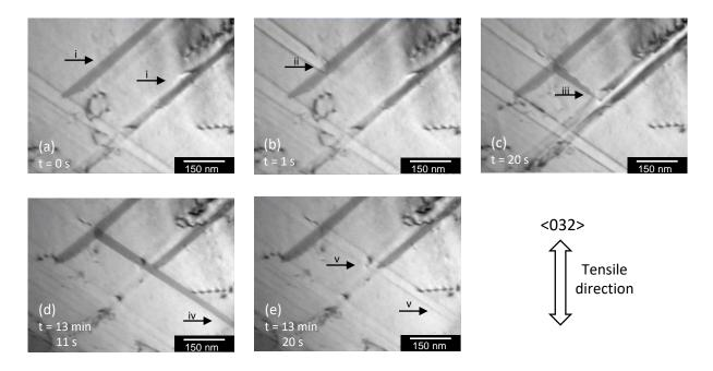
Figure 6: Video sequence showing the nucleation of a stacking fault at 20 °C.
