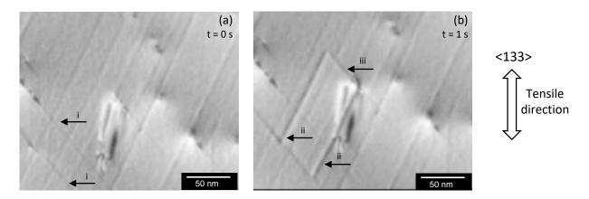
Figure 7: Video sequence of cross-slip at 200°C.
