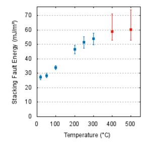
Figure 9: Calculated SFE values as a function of temperature (red dots have a higher uncertainty).
