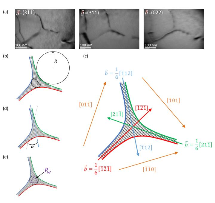
Figure 2: (a) Extended dislocation node under different observation conditions in S-SA at 20°C; (b) Measurement of y and R; (c) Characterization of the dislocations of the node; (d) Measurement of the angle  $\alpha$ ; (e) Description of the perimeter  $P_w$ .
