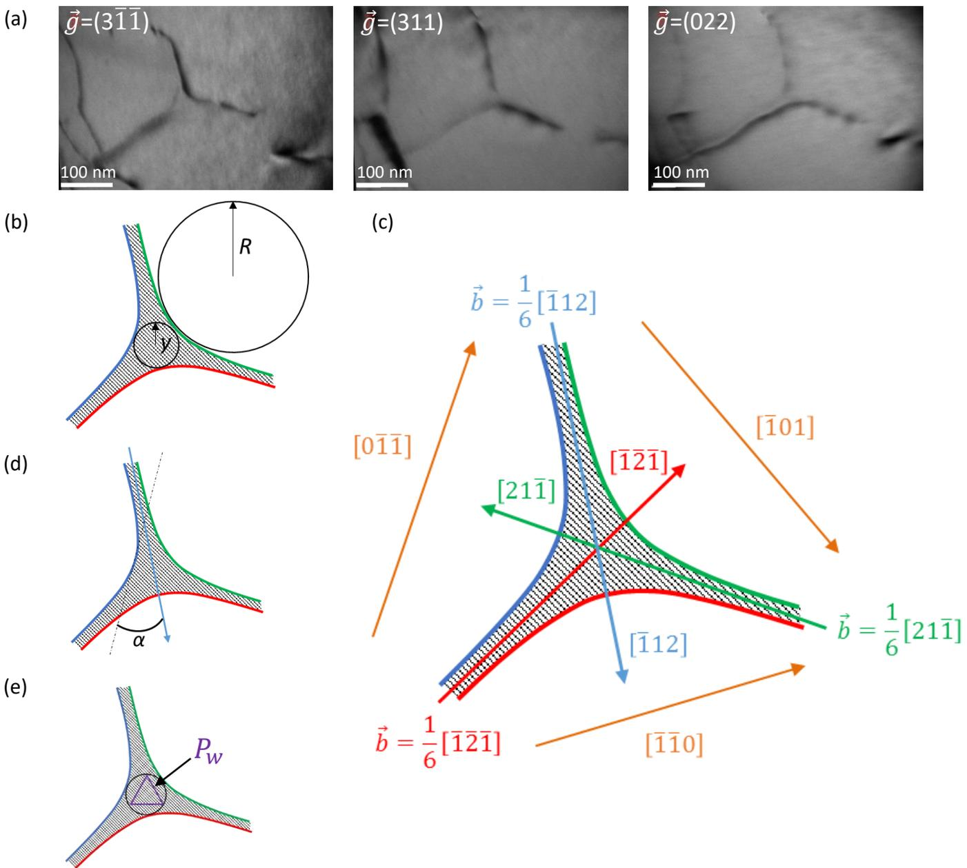
Figure 2: (a) Extended dislocation node under different observation conditions in S-SA at 20°C; (b) Measurement of  $y$  and  $R$ ; (c) Characterization of the dislocations of the node; (d) Measurement of the angle  $\alpha$ ; (e) Description of the perimeter  $P_w$ .
