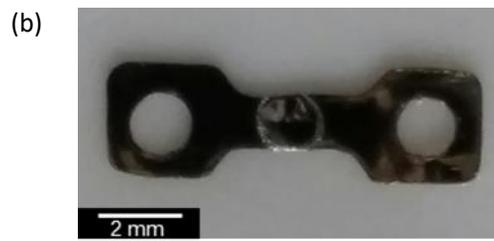
Figure 1 : (a) geometry of a two-leg macro-tensile specimen, (b) geometry of a micro-tensile specimen.
