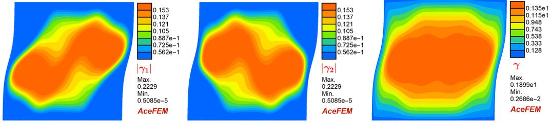
Figure 9: Distribution of slips for  $H = 10 \mu\text{m}$ , final  $\langle \gamma_{xy} \rangle = 0.1$ .
