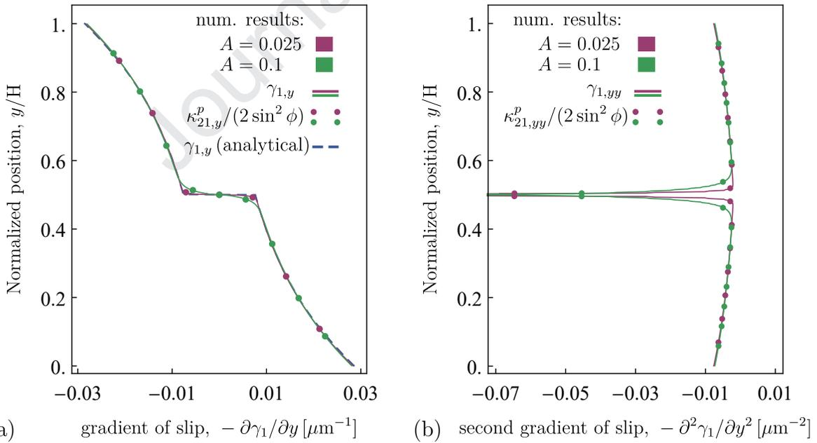
Figure 6: Profiles of the (a) first and (b) second gradient of (local) plastic slip  $\gamma_1$ , and global counterparts  $\kappa_{21,y}^p/(2\sin^2\phi)$  and  $\kappa_{21,yy}^p/(2\sin^2\phi)$ .
