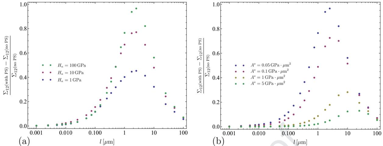
Figure 4: Relative difference  $\frac{\Sigma_{12}(\text{with PS}) - \Sigma_{12}(\text{no PS})}{\Sigma_{12}(\text{no PS})}$  in macroscopic stress at 0.05 average plastic strain in the cases when the P-S term is included or disregarded for (a) various  $H_\kappa$  and fixed  $A^s = 0.05 \text{ GPa} \cdot \mu\text{m}^2$ , and (b) various values of  $A^s$  and fixed  $H_\kappa = 100 \text{ GPa}$ .
