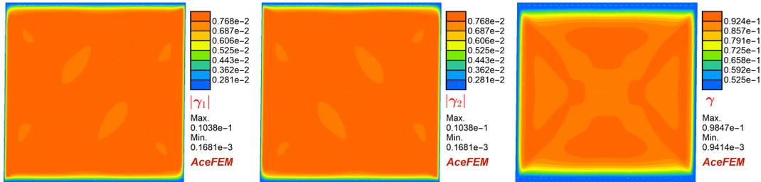
Figure 13: Distribution of slips for  $H = 10 \mu\text{m}$ ,  $\langle \gamma_{xy} \rangle = 0.01$ , P-S term disregarded.
