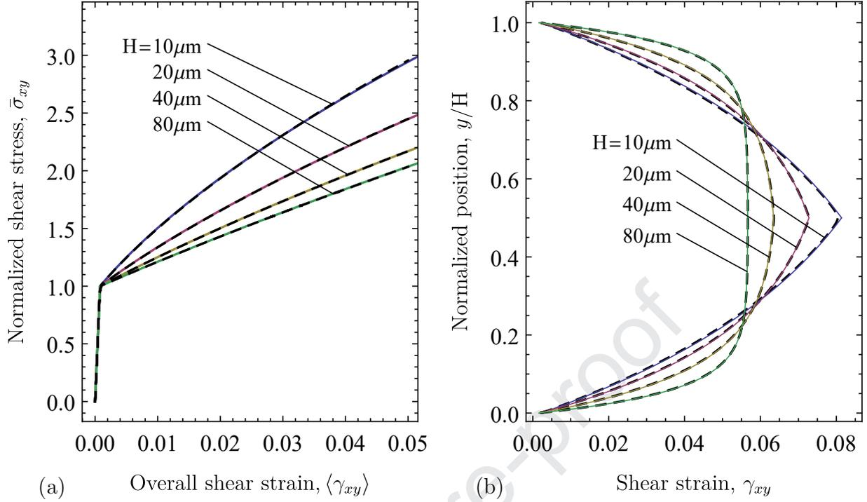
Figure 5: Comparison of the semi-analytical solution of Stupkiewicz and Petryk (2016) (solid lines) with the present FE solution for  $A = 0.1 \text{ GPa}\cdot\mu\text{m}^2$  and  $H_\kappa = 1000 \text{ GPa}$  (broken lines): (a) overall stress-strain response, (b) shear strain profiles for overall shear strain  $\langle \gamma_{xy} \rangle = 0.05$ .
