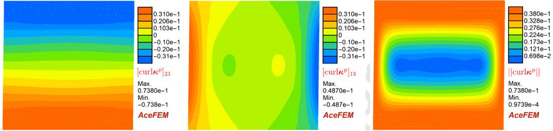
Figure 19: Distribution of the components and norm of  $\text{curl}\kappa^P$  as the GND density tensor, in  $\mu\text{m}^{-1}$ , for  $H = 1 \mu\text{m}$ ,  $\langle\gamma_{xy}\rangle = 0.01$ , P-S term disregarded.
