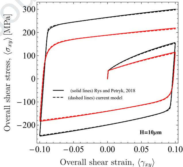
Figure 8: Comparison of the overall stress - overall strain plots for two energy functions of different GND measures for cyclic shear of a square element,  $H = 10 \mu\text{m}$ ,  $A = h_0 L_{\text{en}}^2 = 0.288 \text{ GPa}\cdot\mu\text{m}^2$ . Inner red plots refer to the case when P-S term is disregarded.
