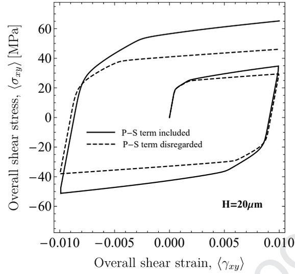
Figure 20: Overall shear stress - overall shear strain plots for the idealized polycrystal.
