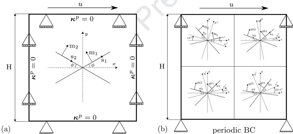
Figure 7: Schematic of shearing of a square element of dimension  $H$ : (a) single crystal and (b) idealized polycrystal.
