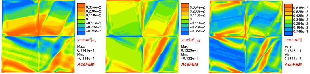
Figure 23: Distribution of the components and norm of  $\text{curl}\kappa^P$  as the GND density tensor, in  $\mu\text{m}^{-1}$ , for  $H = 20\ \mu\text{m}$ , P-S term included.
