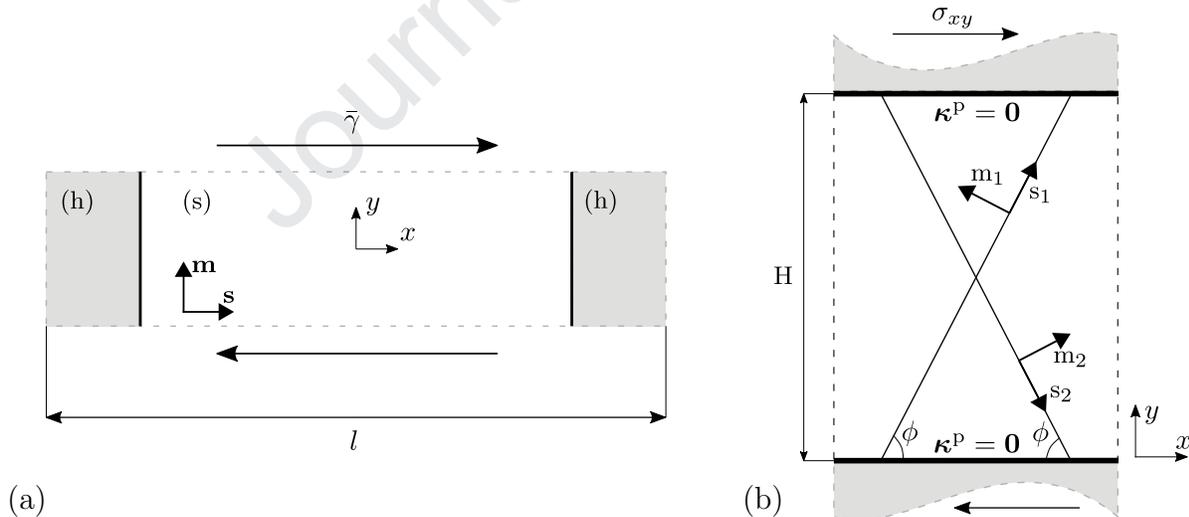
Figure 1: Schematic of the shearing problem: (a) shearing of a periodic single-slip single crystal composed of soft (s) and hard (h) phases, and (b) shearing of a double-slip single crystal.
