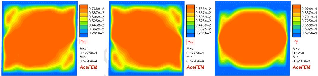
Figure 12: Distribution of slips for  $H = 10 \mu\text{m}$ ,  $\langle \gamma_{xy} \rangle = 0.01$ , P-S term included.
