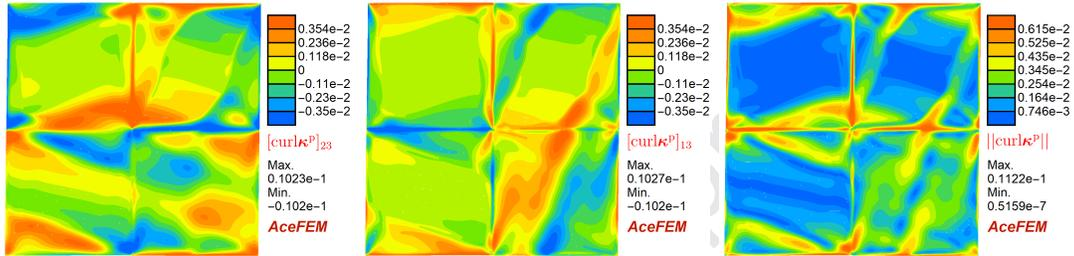
Figure 24: Distribution of the components and norm of  $\text{curl}\kappa^P$  as the GND density tensor, in  $\mu\text{m}^{-1}$ , for  $H = 20\ \mu\text{m}$ , P-S term disregarded.
