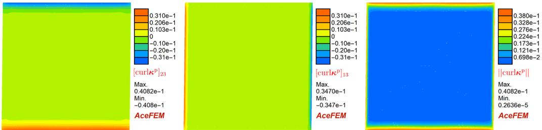
Figure 17: Distribution of the components and norm of  $\text{curl} \kappa^P$  as the GND density tensor, in  $\mu\text{m}^{-1}$ , for  $H = 10 \mu\text{m}$ ,  $\langle \gamma_{xy} \rangle = 0.01$ , P-S term disregarded.
