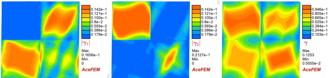
Figure 21: Distribution of slips for  $H = 20 \mu\text{m}$ , P-S term included.
