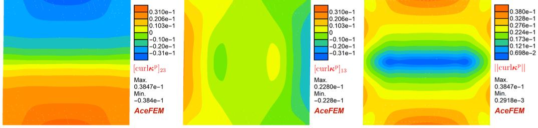
Figure 18: Distribution of the components and norm of  $\text{curl}\kappa^P$  as the GND density tensor, in  $\mu\text{m}^{-1}$ , for  $H = 1 \mu\text{m}$ ,  $\langle\gamma_{xy}\rangle = 0.01$ , P-S term included.
