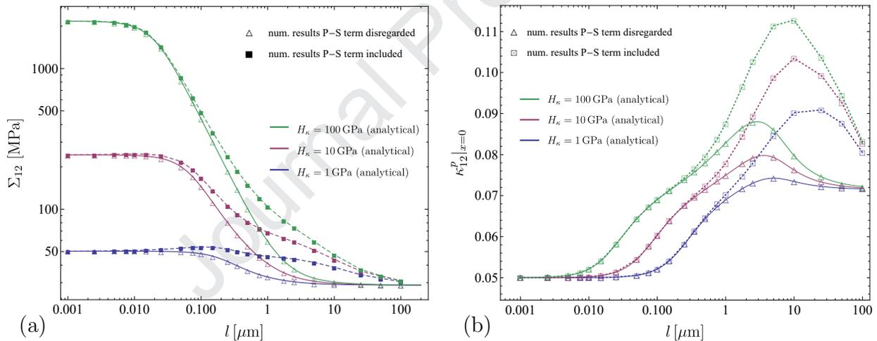
Figure 3: (a) Macroscopic stress  $\Sigma_{12}|_{\gamma=0.05}$  at 0.05 average plastic shear strain as a function of the microstructure length scale  $l$ , computed for  $H_\kappa = 1, 10$  and  $100 \text{ GPa}$  and  $A^s = 0.05 \text{ GPa}\cdot\mu\text{m}^2$  ( $A^h = A^s/100$ ), (b) values of micromorphic variable  $\kappa_{12}^p$  at the center ( $x = 0$ ) of the two-phase laminate.
