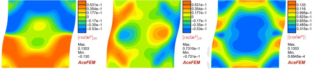
Figure 10: Distribution of the components and norm of  $\text{curl} \kappa^P$  as the GND density tensor, in  $\mu\text{m}^{-1}$ , for  $H = 10 \mu\text{m}$ , final  $\langle \gamma_{xy} \rangle = 0.1$ .
