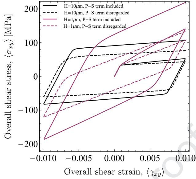
Figure 11: The effect of the P-S term and sample size on the plot of overall shear stress vs overall shear strain in cyclic deformation.
