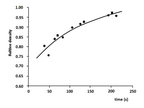
Figure 18. Modelling of the evolution of density during densification (● test 1∎test 2◆ test 3)One can observe that the model reveals well the reality of the densification of this polymer.
