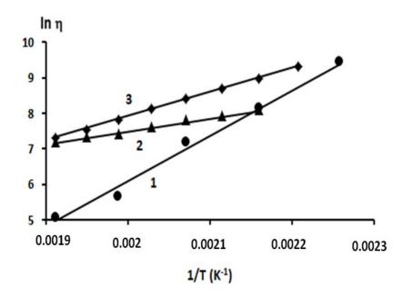
Figure 5. Temperature dependence of viscosity of PP (1), PVDF (2) and PMMA (3).
