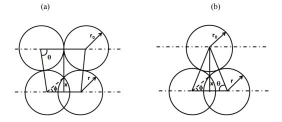
**Figure 3.** Two different arrangements of grains in Bellehumeur model (a) Simple Cubic (SC); (b) Face Centred Cubic (FCC)
