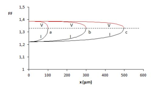
**Figure 14** .Variation of FF versus x for different values of r:  $100\mu m$  (a),  $300\mu m$  (b) and  $500\mu m$  (c). This variation has been plotted for two positions of particle C: I and V.
