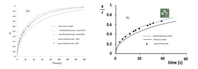
**Figure 15.**Modeling of the coalescence curves for two different grains configuration. (a) PP (b) PMMA.
