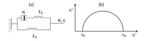
Figure 6. Zener model: schema (a), COLE-COLE Diagram (b)
