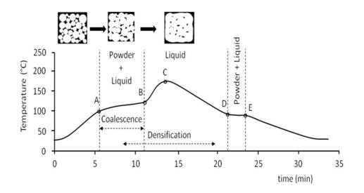
Figure 1. Time-internal air temperature diagram during rotational moulding
