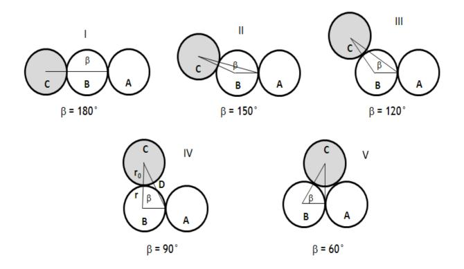
Figure 12.Different position of particle C during the coalescence of grains A and B.
