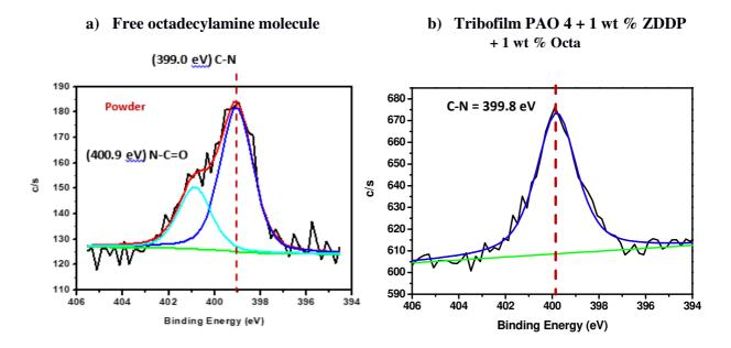
**Figure 10:** High-resolution XPS N 1s spectra of : a) free amine molecule (standard octadecylami). The amide contribution at 400.9 eV is contamination b) the adsorbed octadecylamine on the tribofilm formed in PAO 4 + 1 wt % ZDDP + 1 wt % Octa
