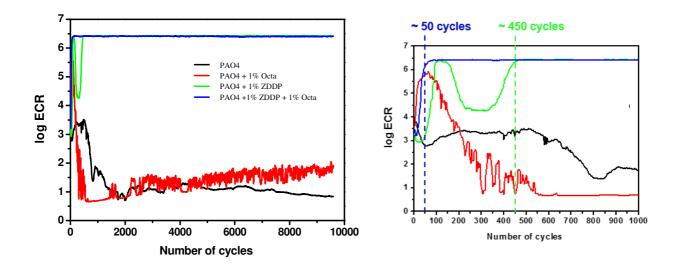
**Figure 7:** (a) Evolution of the electrical contact resistance during friction tests with PAO4, PAO4 + 1 wt % Octa, PAO4 + 1 wt % ZDDP and PAO4 + 1 wt % octa + 1 wt% ZDDP. (b) Zoomed in view of the first 1000 cycles.
