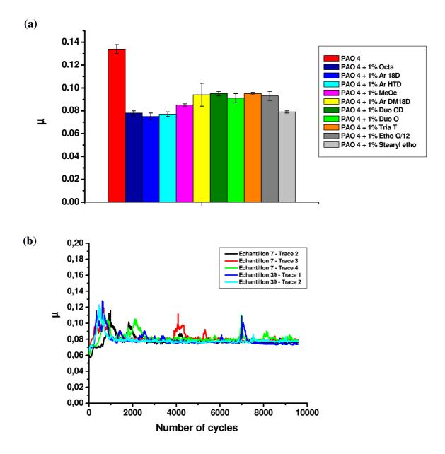
**Figure 2:** (a) Average steady-state friction coefficients  $\pm$  standard deviation obtained at 100°C with and without different types of amines. (b) friction curves obtained for PAO4 +1%octa.
