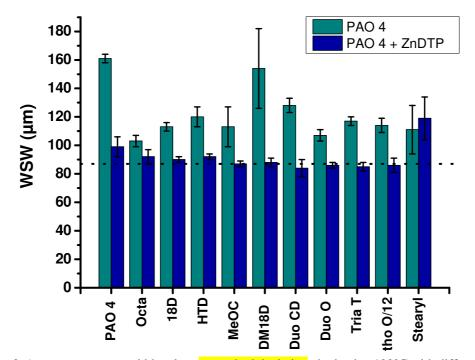
**Figure 6:** Average wear scar width values  $\pm$  standard deviation obtained at 100°C with different blends: in green, PAO4 alone and PAO4 with 1% of different types of amines (binary mixture), in blue, PAO4 + 1% ZDDP and PAO4+1%ZDDP with 1% of different types of amines (ternary mixture). The dotted line represents the calculated Hertz diameter (87 µm).
