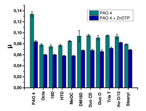
Figure 5: Average steady-state friction coefficient  $\pm$  standard deviation obtained at 100°C with different blends: in green, PAO4 alone and PAO4 with 1% of different types of amines (binary mixture), in blue, PAO4+1%ZDDP and PAO4+1%ZDDP with 1% of different types of amines (ternary mixture).
