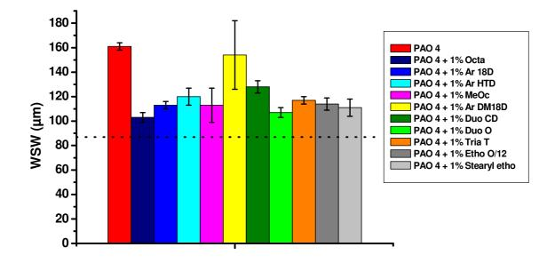
**Figure 4:** Average wear scar width (WSW) measurements  $\pm$  standard deviation obtained at 100°C with different types of amines. The dotted line represents the calculated Hertz diameter (87 µm).
