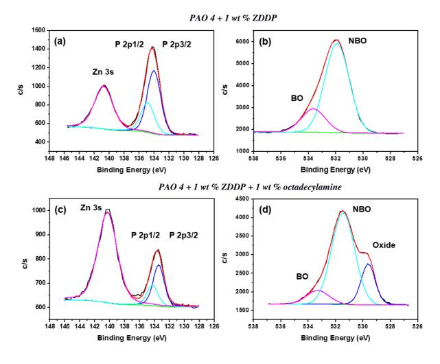
**Figure 9:** XPS spectra of (a) P 2p, Zn 3s and (b) O 1s recorded on the tribofilm formed in PAO 4 + 1 wt % ZDDP. XPS spectra of (c) P 2p, Zn 3s and (d) O 1s recorded on the tribofilm formed in PAO 4 + 1 wt % ZDDP +1% octadecylamine.
