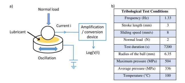
**Figure 1:** Tribological test in reciprocating sliding mode. (a) Drawing showing the working principle of our home-made tribometer allowing to measure simultaneously the evolution of the friction coefficient and the electrical contact resistance as a function of the number of cycles. (b) Experimental conditions used during friction tests.
