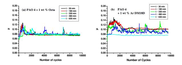
**Figure 3:** Evolution of friction coefficient at 100°C as a function of exposition time "t" e.g. immersion time in lubricant at 100 °C prior to commencing rubbing: (a) PAO 4 + 1 wt % Octa (b) PAO 4 + 1 wt % Ar DM18D.
