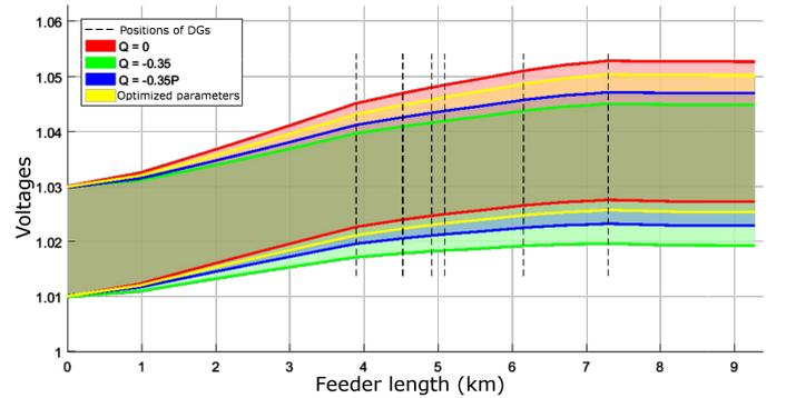
Figure 8. Voltage 95 % confidence levels along the feeder
