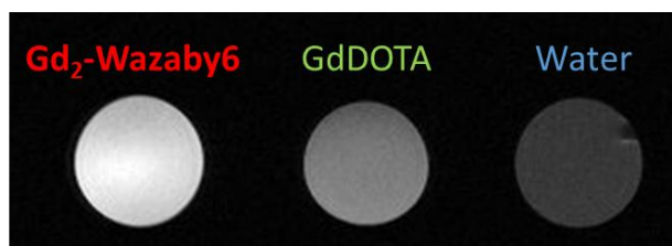
Figure 7: T 1 -weighted MRI phantom images of Gd 2 -Wazaby6 (150 μM), GdDOTA (150 μM) and water (reference) at 7 T using spin-echo sequence with TE = 50 ms and TR = 500 ms.
